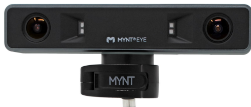
Figure 2.1 – Example of stereo + depth camera with an embedded IMU, a MYNT EYE D1000-120, the camera we used to create our datasets. Image from the MYNT EYE company website.
