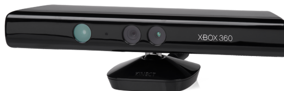
Figure 2.3 – Example of RGB+depth camera, a Kinect, often used in SLAM benchmarks. Image from Wikipedia.
