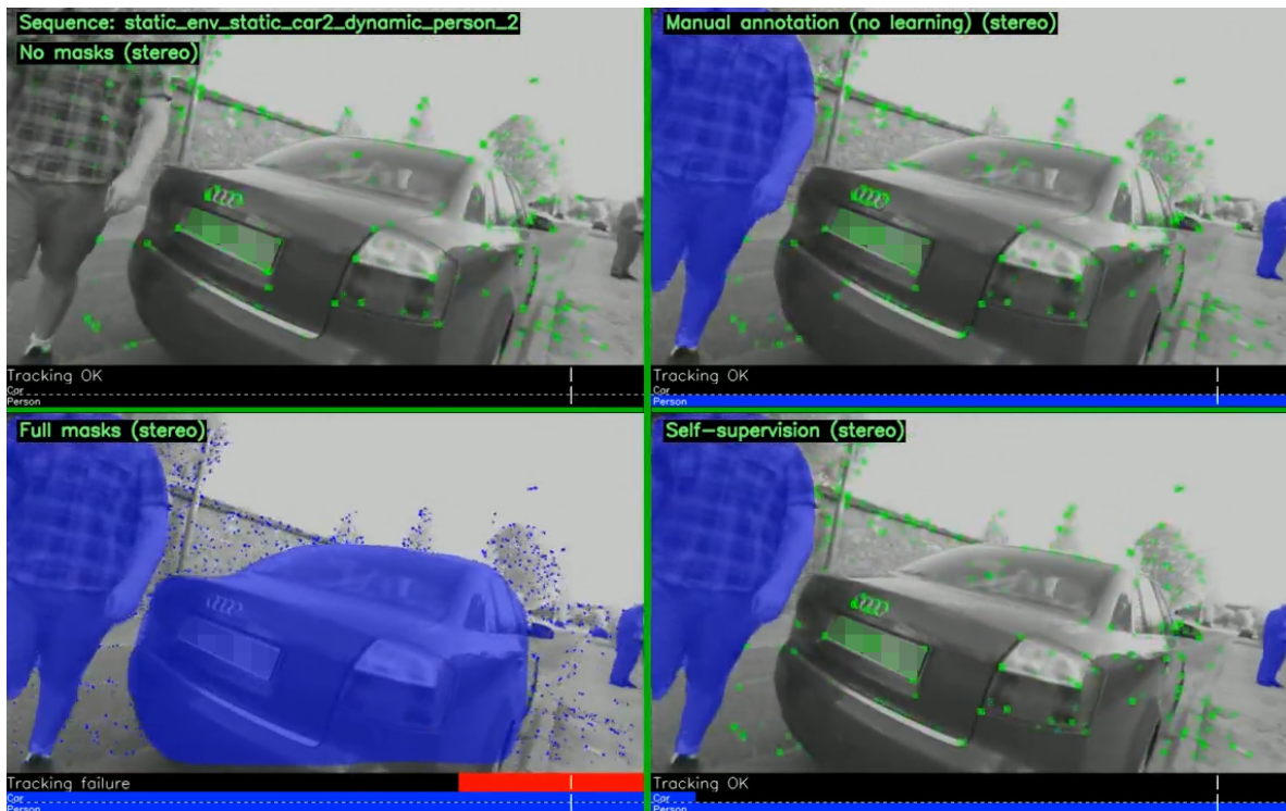
(a) Masking result on a difficult sequence with moving people and static cars. Our approach masks people all the time and almost never cars, making the inferred annotation and the manual annotation very similar.
