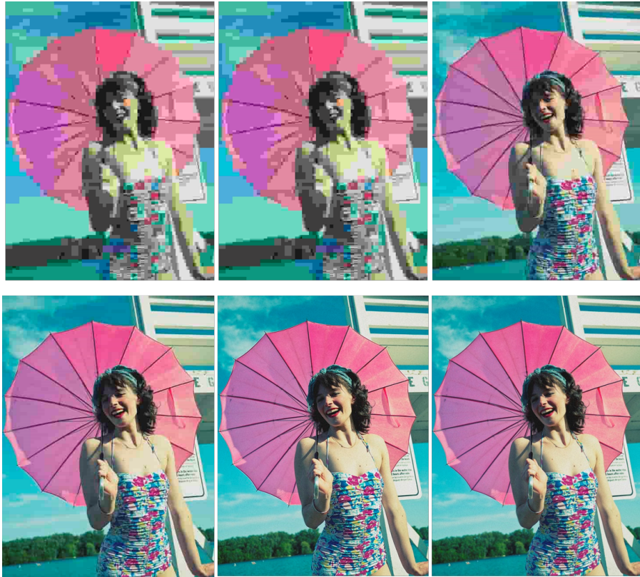
Figure 3.13 – Examples of images of degraded quality using various levels of JPEG compression.
