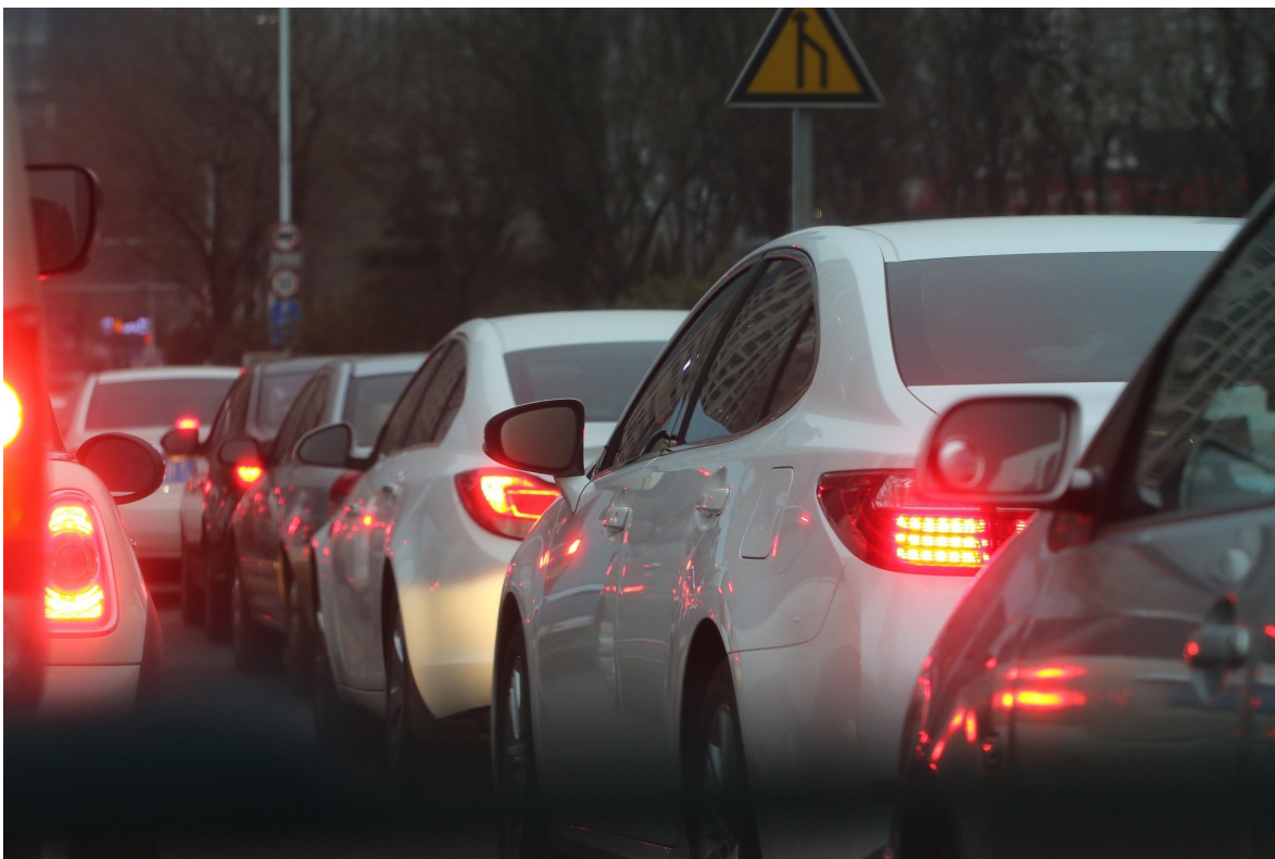
Figure 1.2 – Example of dynamic scenario difficult for a SLAM algorithm, a traffic jam. The motion consensus (the dominant motion) does not correspond to the ground but to the motion of cars.
