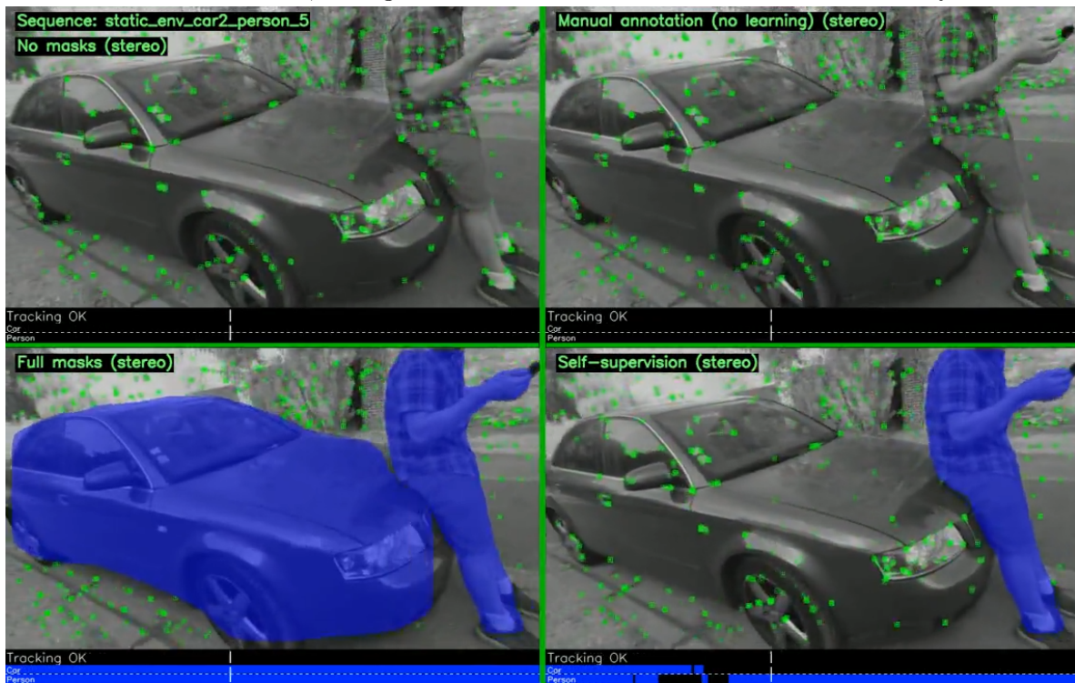
(b) Masking result on a sequence where both people and cars are static. Our approach is more prudent towards masking, but correctly stops masking when needed. Blue segments indicate masked frames, per class.
