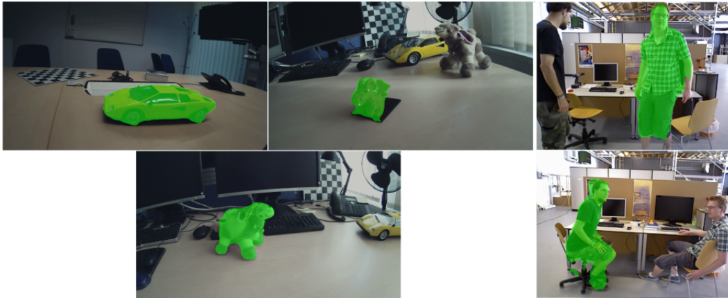
(a) We detect and mask the dynamic objects of monocular sequences (left: our dataset, right: TUM RGB-D).
