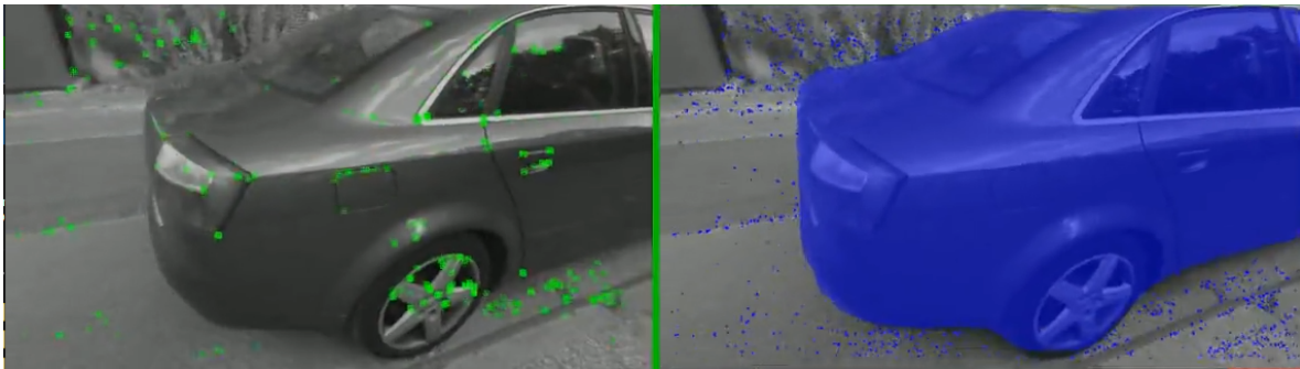
(a) Excessive masking in the ConsInv-Outdoors with a static car. In the right figure, most features are removed by masking the car, leaving not enough of them for the SLAM to work and causing it to fail.
