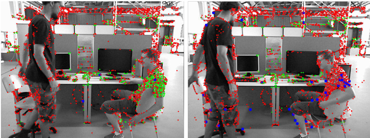
Figure 3.20 – Scene before and after a person gets up (10 frames apart). Red: unmatched features, green: matched features (inliers), blue: outliers. We see that all inliers on the sitting person vanished and were replaced by either unmatched features or outliers.
