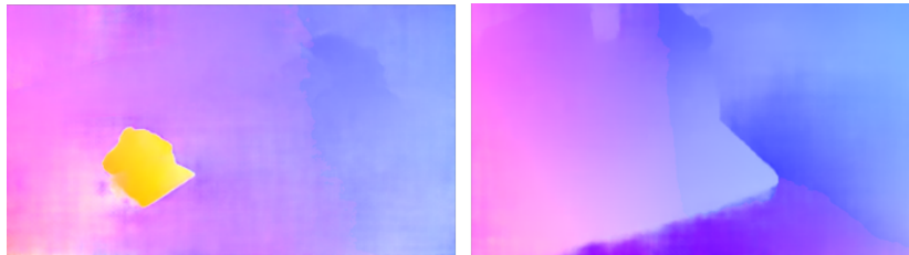
Figure 2.14 – Example of optical flow using PWC-Net [91]. The camera and the object are both moving in the two images. The object is far from the camera in the left image and close to it in the right one.
