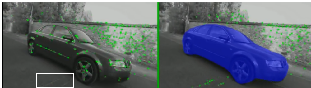
(a) Severe MCI in the ConsInv-Outdoors dataset with a moving car. In the left figure, useful features on the ground are missing while the majority of features is on a moving car, which causes SLAM drift.
