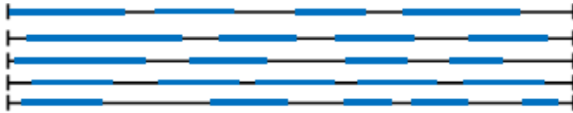
Figure 6.6 – Illustration of sampled temporal masks from a temporal mask space (blue = masked, black = not masked). Conditions k_0, k_1 on masked/unmasked block sizes prevent quick changes between masking states.
