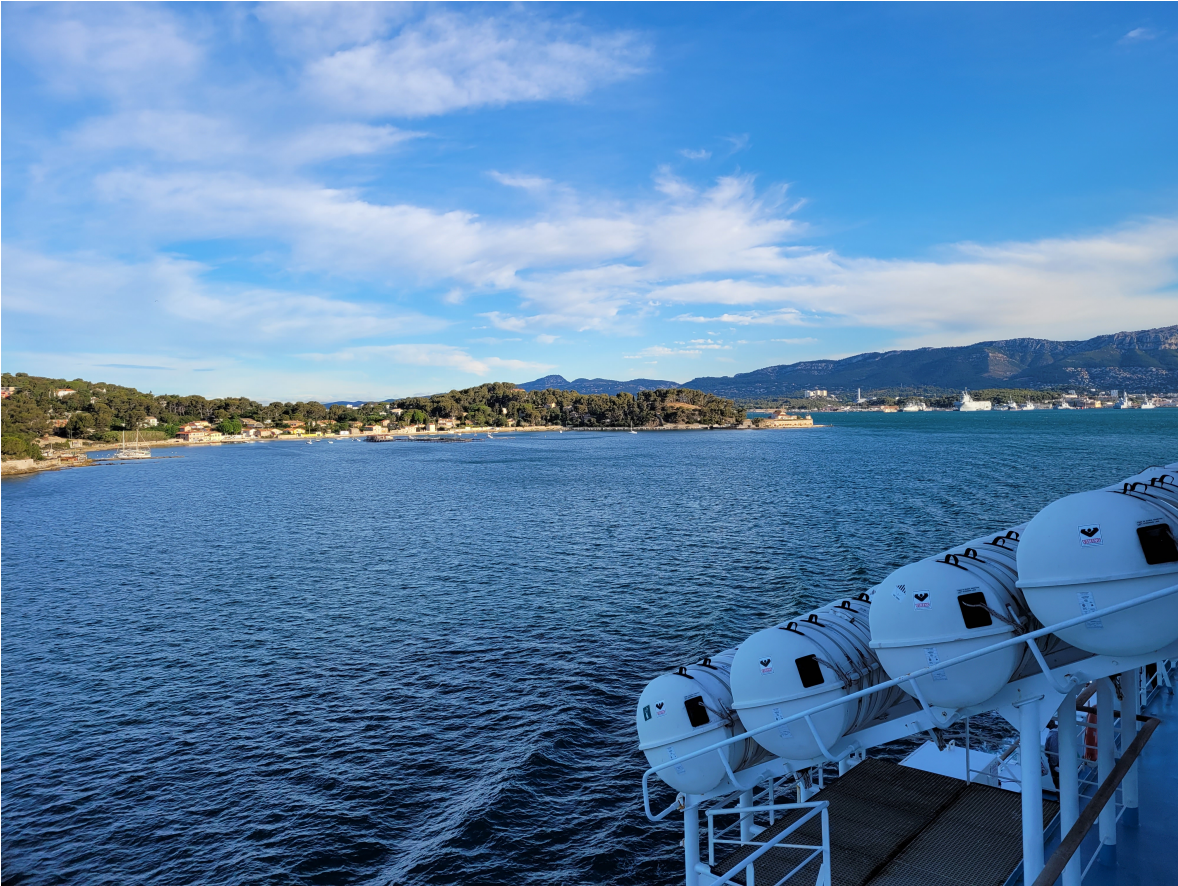
Figure 1.3 – Example of very difficult dynamic scenario for a SLAM algorithm. The frame of reference that the user wants to use for localization is not obvious: it could be the Earth or the ship itself. There is no clear consensus in the image: the sky, the sea, the Earth, and the ship move differently.
