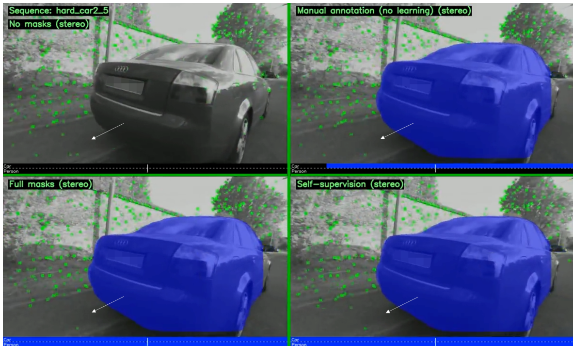
(b) Masking result on a difficult sequence with moving cars and no people. Our approach says to mask both people and cars all the time out of caution.
