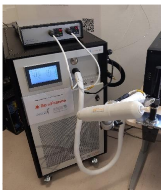
Figure 2.1: PTR-Qi-TOF MS with a buffered-end tidal device (BET med, Herbig et al. 2008 ), Exhalomics, Foch Hospital.
