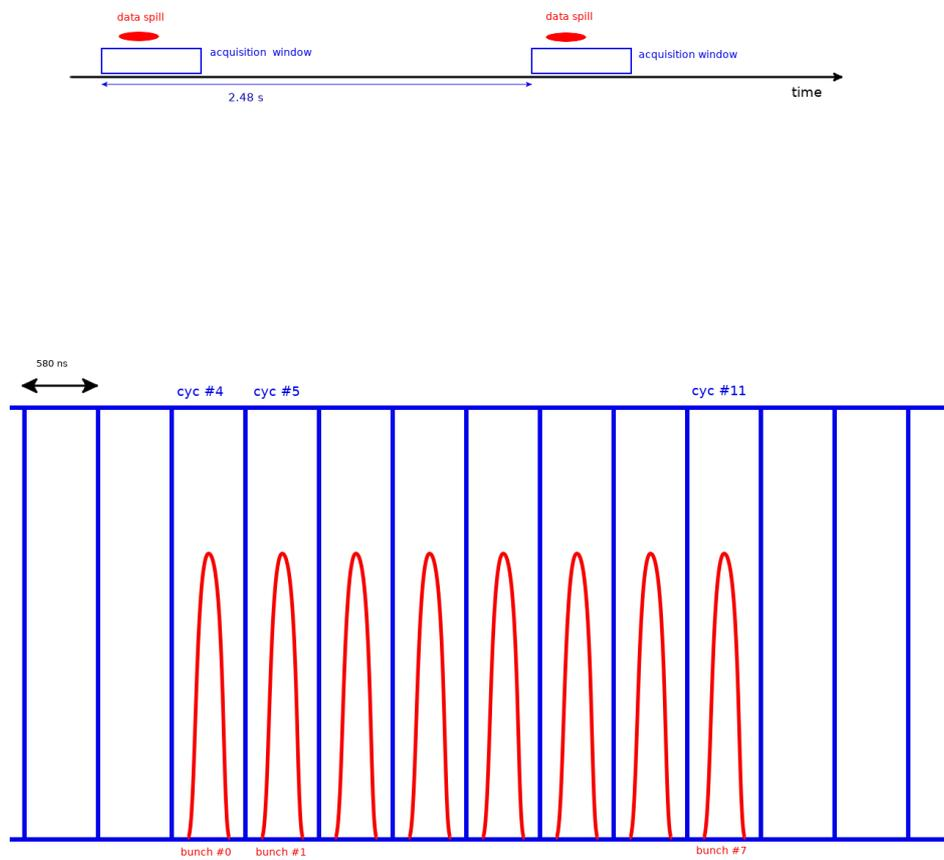
Figure 3.12 – Data acquisition. Superposition of the neutrino spill and of the acquisition window (top). Synchronization of the 8 bunches of the spill with the 23 cycles of the acquisition window (bottom)
