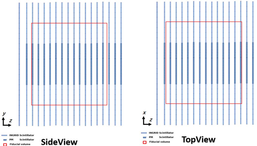
Figure 3.14 – Fiducial volume for the Proton module. For side view (left) and top view (right).
