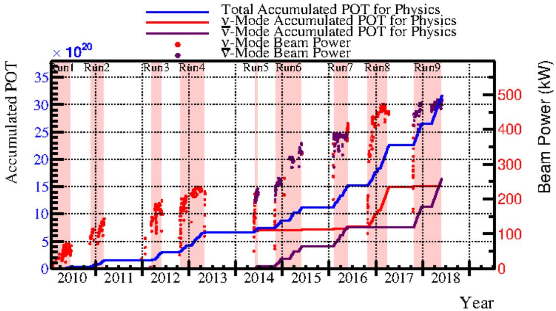
Figure 7.1 – The accumulated POT over the years in the T2K experiment from 2010 to 2018. The POT total can be read on the left vertical axis while the power of the beam can be read on the right vertical axis.
