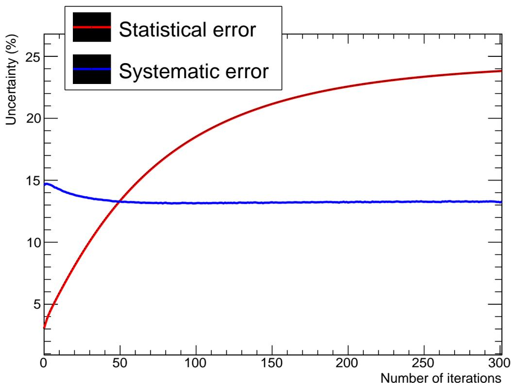
Figure 6.1 – The evolution of the systematic and statistical errors on the total water cross-section  $\sigma_{H_2O}$  with the unfolding step. The systematic error converges while the statistical error increases. The systematic error regroups the errors from the cross-section model, flux and detector response uncertainties.
