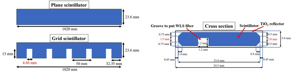
Figure 3.4 – Geometry of the WAGASCI scintillators in the Monte-Carlo
