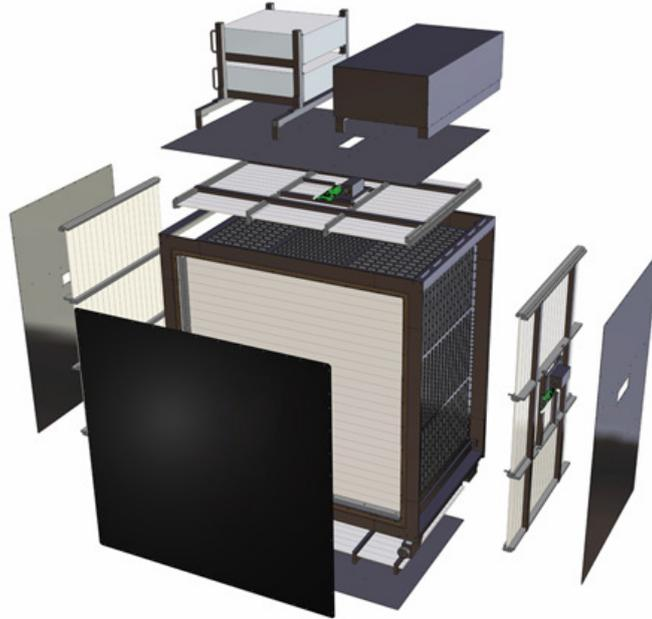
Figure 2.24 – Internal structure of the Proton Module.
