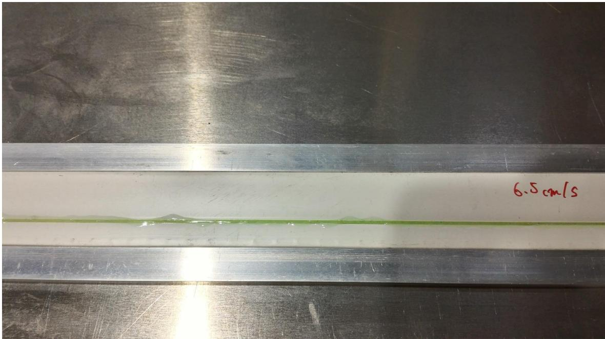
Figure C.2 – Scintillators after the gluing procedure. The amount of optical cement has been dispensed uniformly over the fiber.
