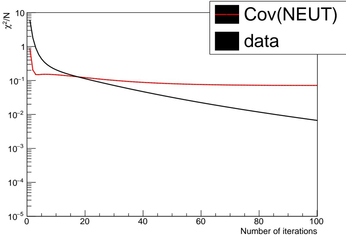
Figure 6.6 – Convergence of the unfolding of the CH selection for fake data#1
