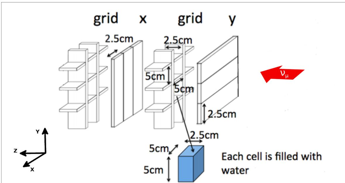
Figure 2.18 – One block of the Water module
