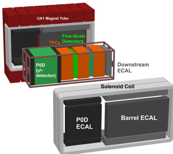
Figure 2.11 – Scheme of the ND280 detector.
