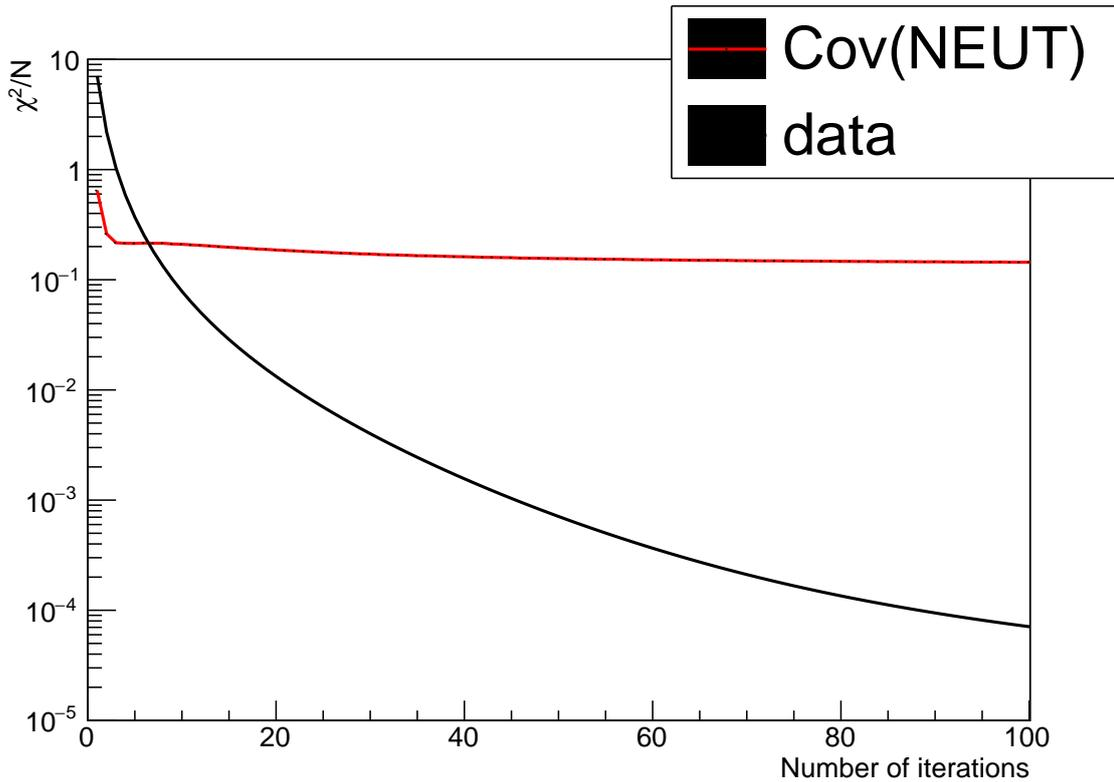
Figure 6.5 – Convergence of the unfolding of the H<sub>2</sub>O selection for fake data#1
