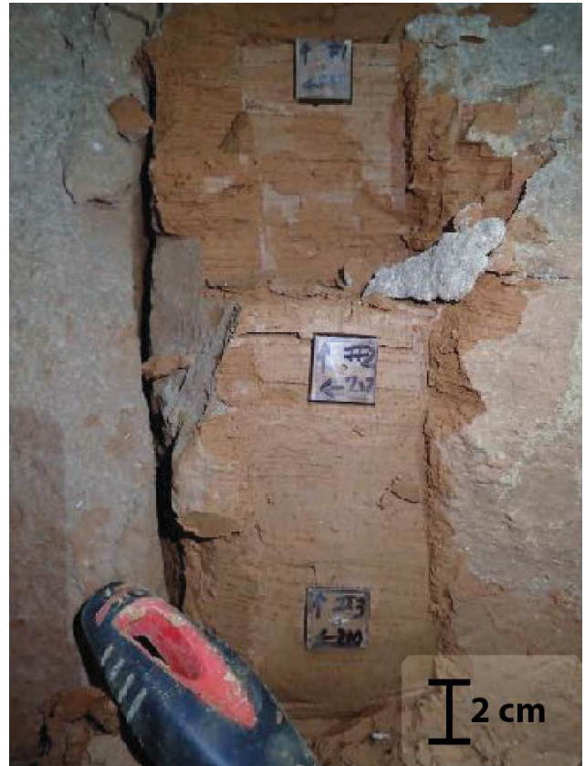
Figure 4. Example of clay sampling for the paleomagnetic study. Location at the entrance shaft (highest elevation of every samples, \sim 580 m a.s.l.; Leicasse cave system, Site 2, Fig. 1).
