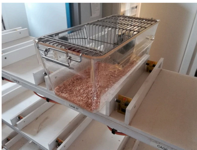
Figure 21. Actigraphy set up. Cage and location of two lasers at each end.
