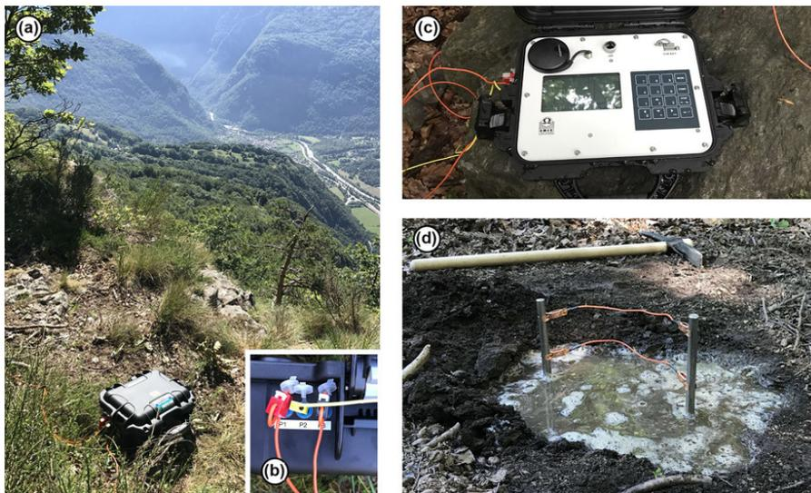
**Figure 3.** Photographs of the monitoring equipment and of the measurement sites: (a) V-FullWaver unit at position FW9. (b) Zoom on the plugs for the three measurement channels on a V-FullWaver unit. (c) Zoom on the control screen of a V-FullWaver unit. (d) Remote electrode fully watered with a highly conductive salted mixture.
