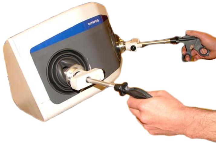
Figure 1.13: View of the operator interface of the EndoSAMURAI. The movement is transmitted mechanically from the interface to the distal part. [Spaun et al., 2009b].
