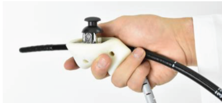
Figure 1.19: Controller of the easyEndo being held together with a conventional endoscope [Lee et al., 2019].
