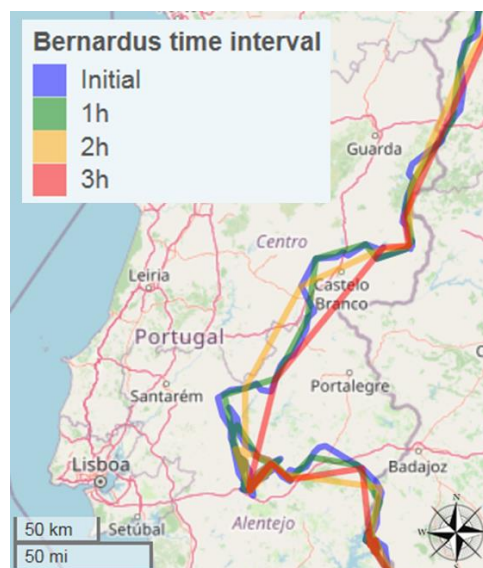
Figure 3: Bernardus trajectory according to different GPS sampling frequencies (initial time interval, i.e. 1 second; 1 hour; 2 hours; 3 hours). A sampling frequency of 1h appears to catch a substantial level of details of the real trajectory.
