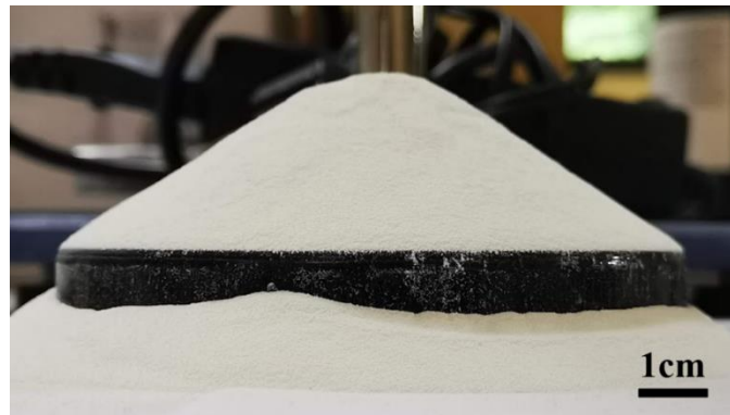
Figure 143. Scheme of artificial angle of repose measurement
