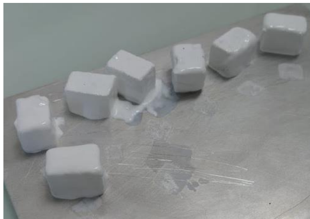
Figure 98. Samples infiltrated with viscous suspension containing 70 wt% solid loading
