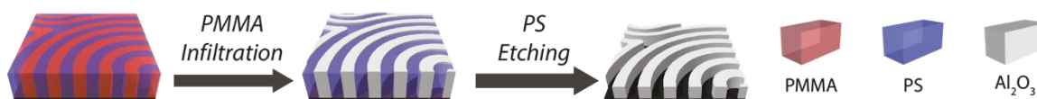
Figure 55. Schematics of the PMMA infiltration followed by a PS etching process for out-of-plane lamellae.
