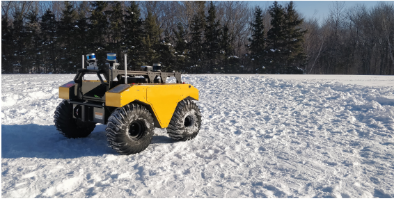
Figure 2.16: Example of terrain where deterministic prediction of the robot's displacement would fail: because of the snow, the robot's skidding and slipping are almost impossible to estimate accurately.
