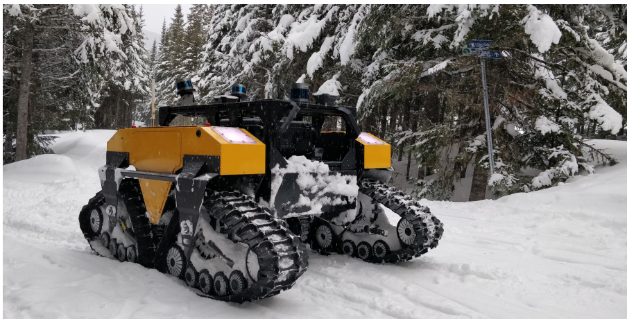
Figure 5.1: Example of unstructured environment where semantic maps would have trouble mapping all the potential obstacles. The snow banks, trees and vegetations lead to a very unstructured environments with no clear features that a semantic mapper could use.
