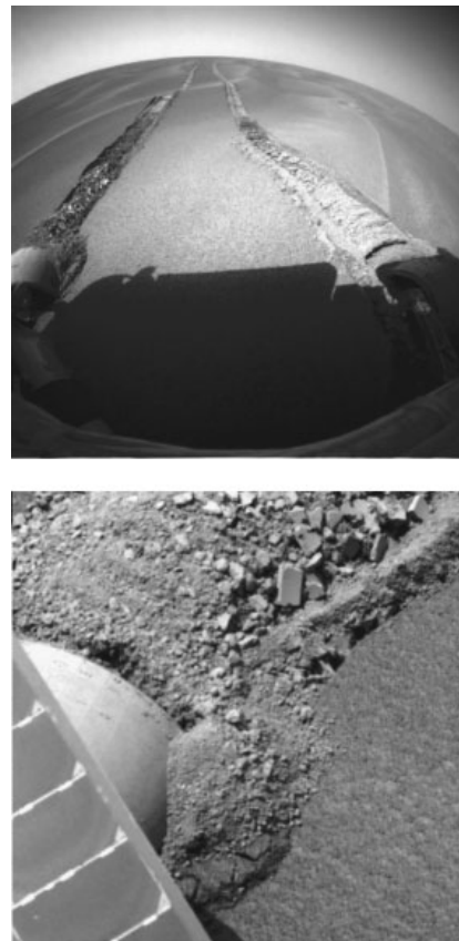
Figure 2.5: Example of hazardous terrain in the context of space robotics. The rover Opportunity is trapped in the Purgatory dune on sol 447. More than five weeks were required to get the rover out of the dune. Image credit: NASA/JPL.
