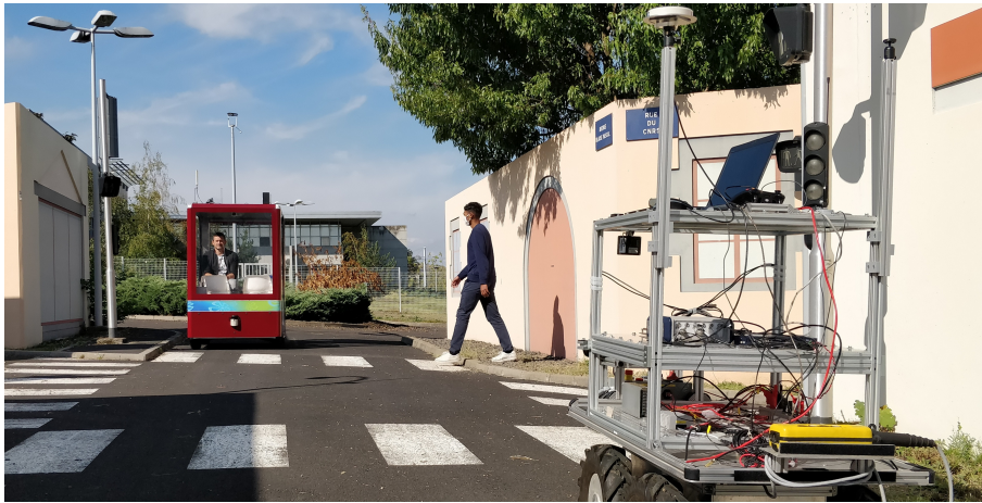
Figure 2.13: Example of scenario a mobile robot might encounter, from [80]. In this case, a ‘risky’ event is the robot colliding with either the pedestrian or the other vehicle.
