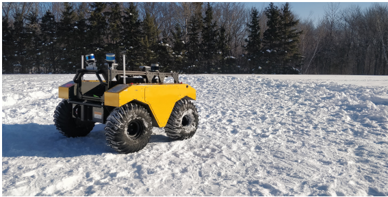
Figure 2.16: Example of terrain where deterministic prediction of the robot's displacement would fail: because of the snow, the robot's skidding and slipping are almost impossible to estimate accurately.
