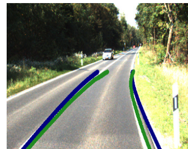
Figure 3.3: Example of lane detection for topological road mapping with a lidar (green) and a camera (blue), from [145].
