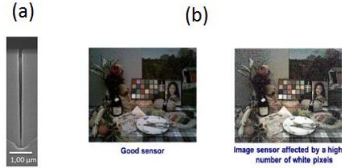
Figure I.16 Cross-sectional SEM image of DTI (a), white pixels phenomenon appearing on defective sensor (b) [10].
