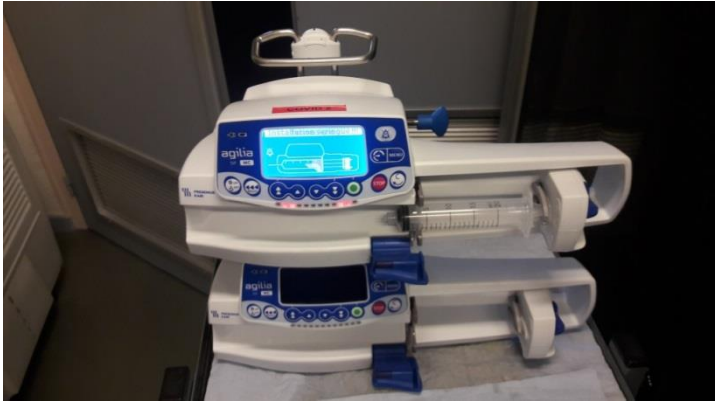
Figure III.32 Syringe pump used to inject liquid at different flow rates
