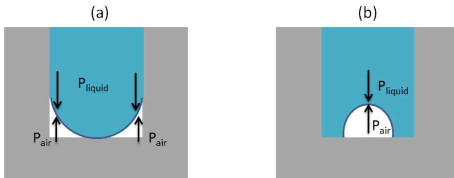
Figure IV.22 Pressure equilibrium between trapped air pockets and suspended liquid inside the DTI for (a) hydrophobic surface and (b) hydrophilic surface
