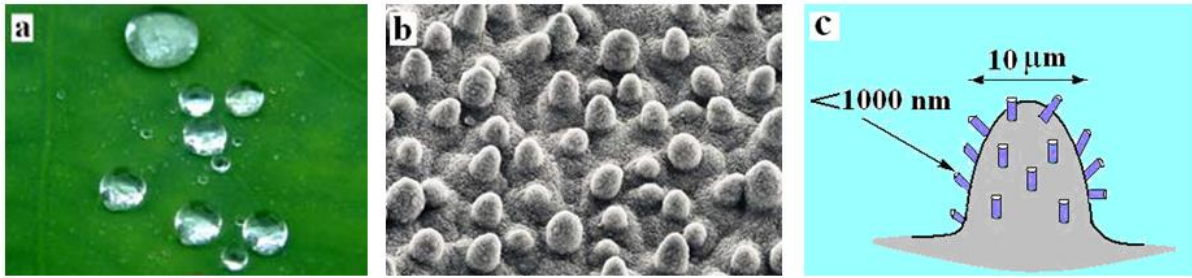
Figure.2 Liquid droplets suspended on lotus leaf (a), SEM image of micro-textured surface of the leaf (b) and (c) micro/nanostructure of the lotus leaf surface [2]
