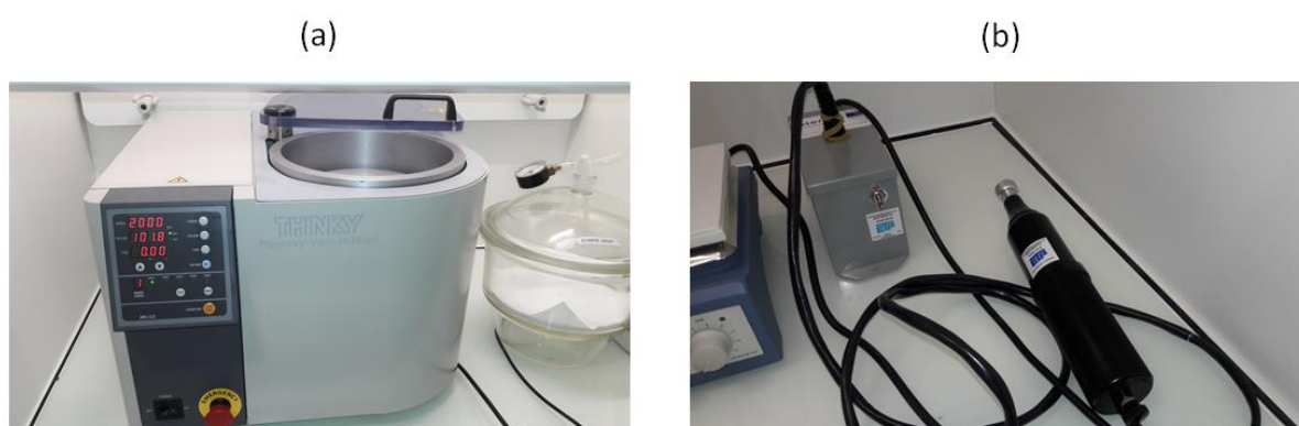
Figure III.28 Photograph of Thinky mixer used to prepare the PDMS (a) and plasma O 2 equipment used to bond the PDMS micro-channel to the DTI silicon sample (b)
