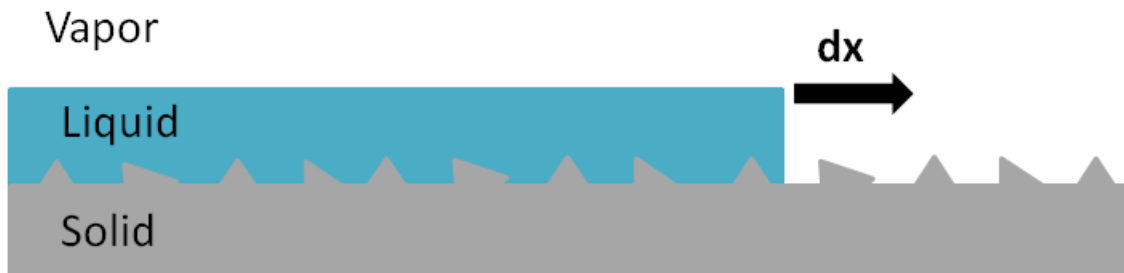
Figure I.4 Infinitesimal displacement of the contact line in Wenzel case
