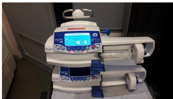
Figure III.32 Syringe pump used to inject liquid at different flow rates
