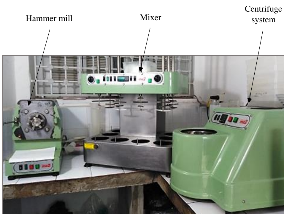
Figure II.3: The Abencor system (OTIT).
