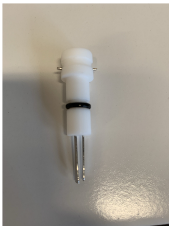
Figure 2.10: Image of a home made PTFE electroformation cap with platinum electrodes. The gap between the electrodes was about 2.5 mm.
