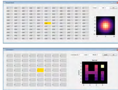
Figure 8: The kernel window allows the setting and drawing of the kernel that will be employed for image convolution. Top: Gaussian kernel, bottom: custom kernel.
