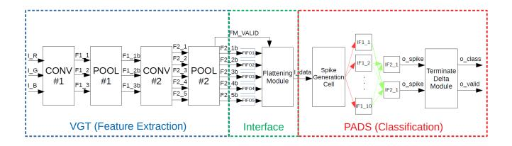
Figure 6.9: Illustration of the CIAR Hybrid Neural Network Architecture.
