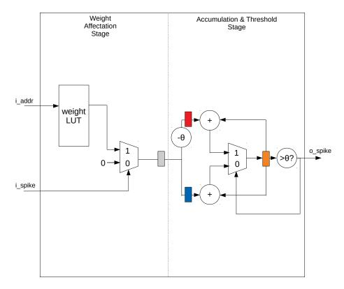
Figure 3.5: Architecture of a PADS Input-NPU, optimized for the input FC layer
