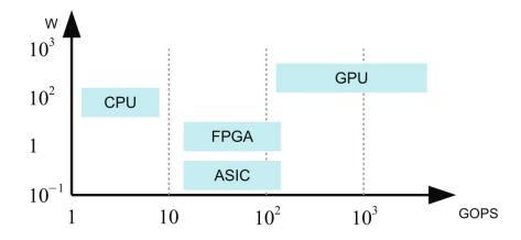
Figure 2.4: Summary of comparisons between CPU, GPU, ASIC and FPGA for neural network acceleration in terms of power consumption and computing power [2].
