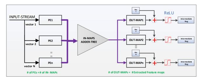
Figure 2.7: Illustration of a VGT-generated convolution layer architecture [5].
