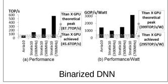
Figure 2.6: Comparison of FPGA (Stratix 10) and GPU (Titan X) for Deep Neural Networks in terms of performance and performance per Watt, for various optimizations: pruning, compact data and binarization. [4].
