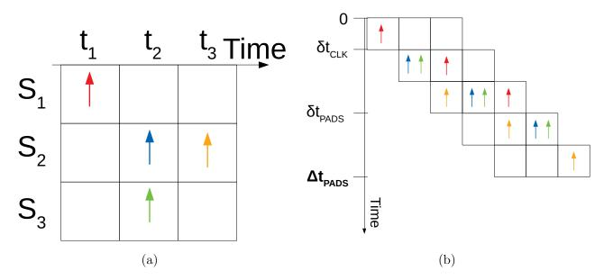
Figure 5.7: a) Simple spike trace example with 4 input synapses and 4 time increments, b) Illustration of PADS parallel and pipelined process.
