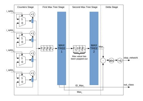
Figure 3.6: Architecture of the PADS' Terminate Delta Module with 4 output neurons.
