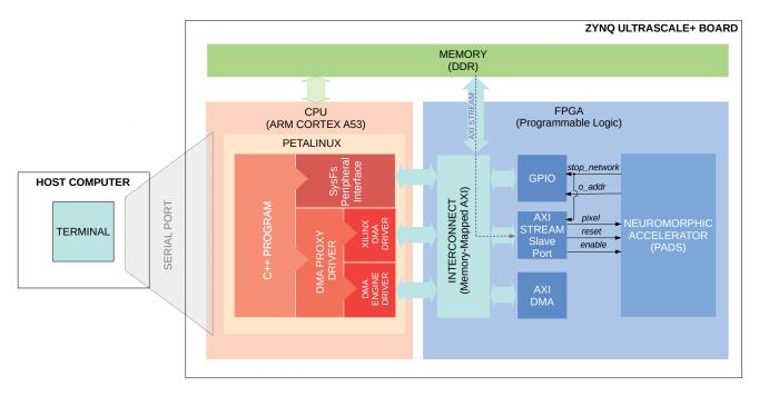
Figure 2: Custom FPGA platform for neuromorphic accelerator deployment. The software stack is in shades of red, and the hardware stack is in shades of blue.
