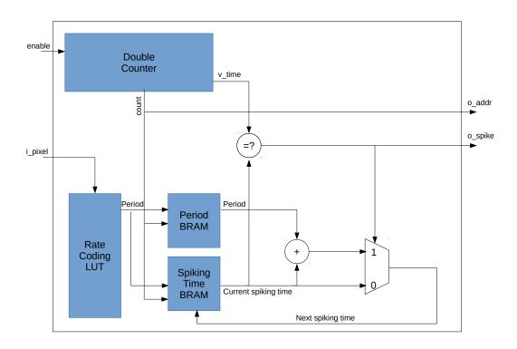
Figure 3.2: Block Diagram of the Spike Generation Cell.
