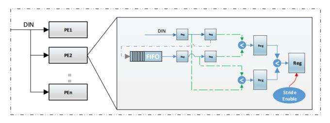
Figure 2.9: Illustration of a VGT-generated max-pooling layer architecture [5].
