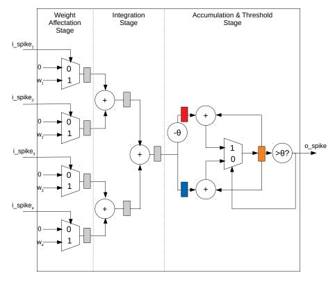
Figure 3.4: Architecture of a generic NPU in PADS, represented with 4 input synapses. Register barriers are represented as rectangles.
