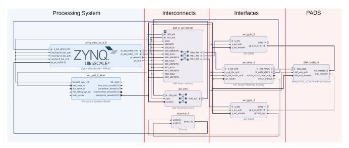
Figure 3: Vivado block design of the FPGA part of the SNN deployment platform.
