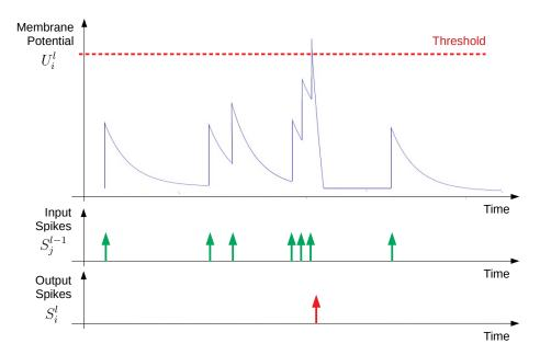
Figure 7.2: Illustration of the Leaky Integrate & Fire neuron process. The membrane potential is shown in blue, input spikes in green and output spikes in red.
