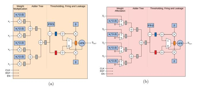
Figure 7.4: Hardware architecture of: a) FISO neuron with 4 input pixels, b) LIF neuron with 4 input synapses. Register barriers are shown in gray or colored rectangles. Data stored in memory is depicted in light blue squares.
