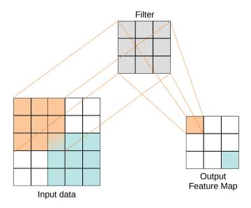
Figure 2.2: Schema of a Convolutional layer, with a 5x5x1 input data, a single 3x3 filter and a stride of 1.
