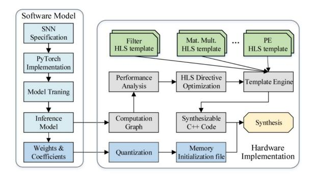
Figure 2.17: Illustration of the training, compression, conversion and hardware deployment framework proposed in [11].
