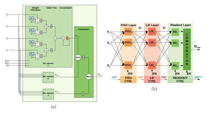
Figure 7.5: a) Architecture of the Readout layer with 4 input synapses and 3 neurons. b) Overview of the full architecture of PADS V2.
