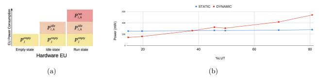
Figure 5.9: a) FPGA power consumption model, b) Dynamic and Static power VS LUT occupation (%) on Zedboard
