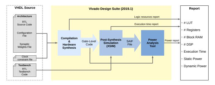
Figure 3.7: Workflow for synthesis, simulation and reporting using Vivado Design Suite (2019.1). The source code (VHDL) is depicted on the left, and the resulting report on the right.
