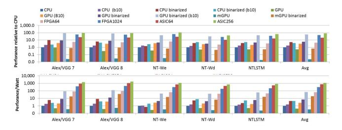
Figure 2.5: Comparison of CPU, GPU, ASIC and FPGA for binary neural network acceleration in terms of speed and performance per Watt, on various neural network topologies [3].
