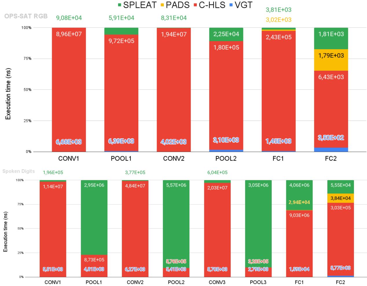
Figure 5.14: Layer-wise execution time (per image) estimation in VGT, HLS, PADS and SPLEAT. Top: OPSSAT RGB, bottom: Spoken Digits
