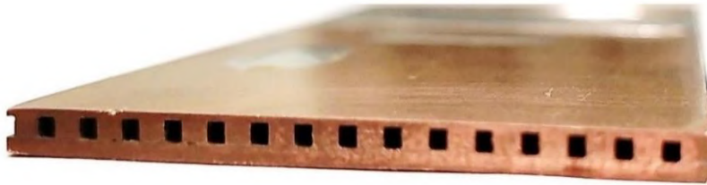
Figure 5.7. Cross-section cut of a welded flat plate PHP sample.
