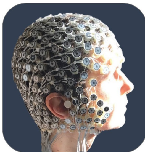
Figure 4. High-Density EEG system (EGI, 256 electrodes) used in Study III
