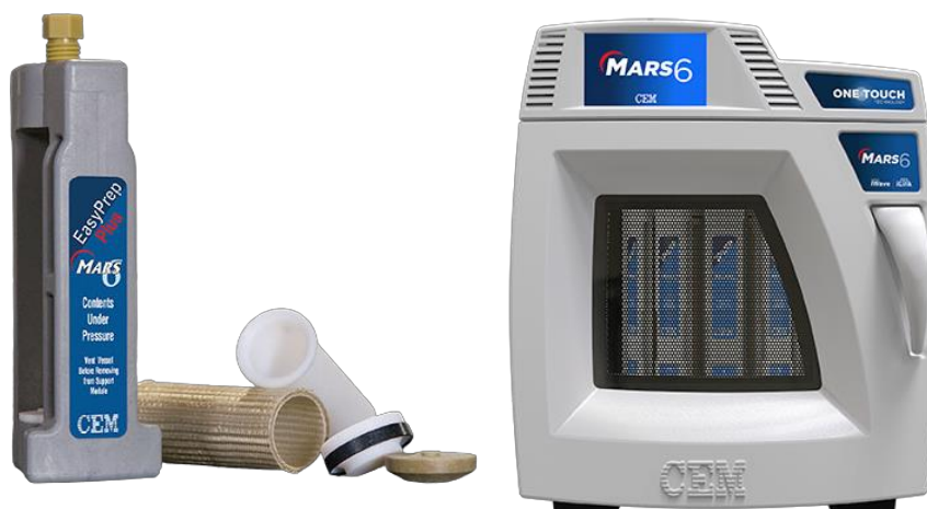
Figure II-3 : Photograph of a single Teflon-lined reaction vessel (EasyPrep Plus) and the microwave synthesizer Mars 6 equipped with multiple vessels (Copyright CEM Corporation).
