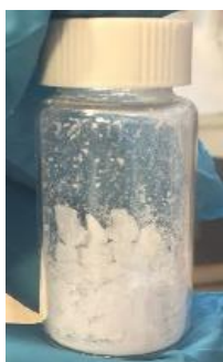
Figure A.-2 : Photograph of the activated MOF-5. The activated sample was stored in the Ar glove box without any exposure to the air.
