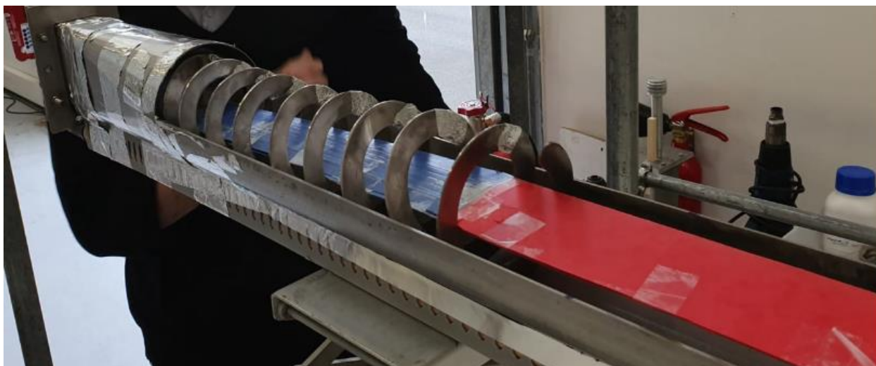
Figure 2.5-4. Placement of thermal paper inside the cavity
