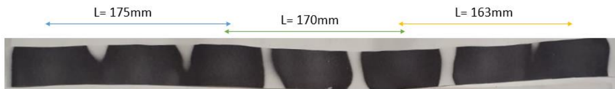
Thermal paper inside the empty reactor irradiated by 15 seconds with a incident power of 600 watt. Length 60mm
