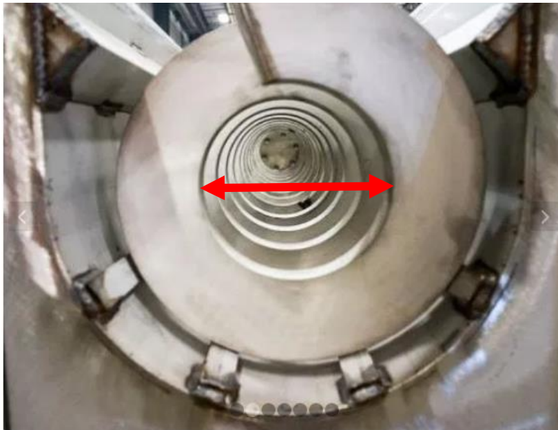
Figure 5.1-2 Shaftless spiral/screw internal diameter
