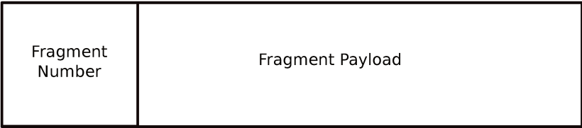
Figure 5.15: A LoRaWAN payload with a single fragment.
