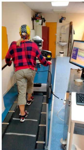
Figure 1. EEG recording during treadmill walking in a healthy subject. The EEG system is synchronized with a video-based motion analysis system (retroreflective markers on both feet) that allows recording of the different events (foot off and strike) characterizing gait. Cortical activity was recorded with an Ag/AgCl 128-scalp-electrode cap (Waveguard®, ANT Neuro, Enschede, The Netherlands). Data were acquired with ASA™ software (ANT Neuro).
