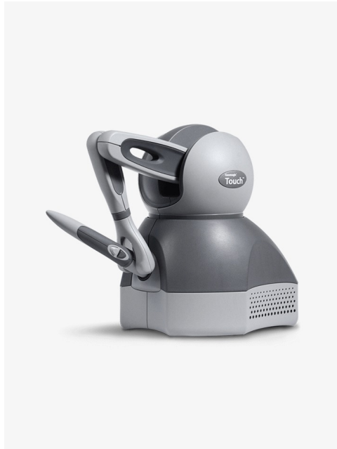
Figure 2.3: The Geomatic Touch haptic arm [126].
