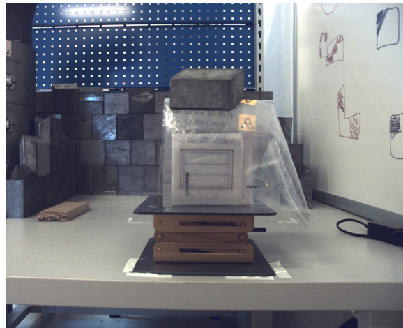
Fig. 3.9: Planar ^{57}\text{Co} source of size 7 cm \times 5.5 cm with activity of 429 kBq at 50 cm from the gamma camera, providing an ambient dose equivalent rate of \sim 340 nSv/h at the measurement point.
