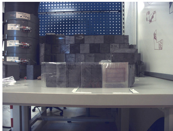
Fig. 3.21: Combination of six planar ^{57}\text{Co} sources with 1716 kBq of total activity.
