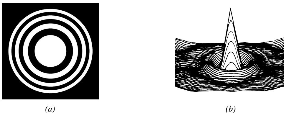
Fig. 1.5: (a) A Fresnel Zone Plate (FZP) pattern with three opaque rings and (b) its autocorrelation function [46].
