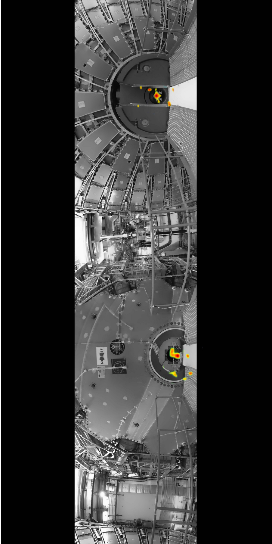
Fig. 3.29: A panorama image with size 8494 \times 1903 pixels, with an horizontal and vertical FOV respectively of 360^\circ and 80^\circ , resulting from the stitching of 120 optical images and the superimposition of 2 \gamma -images. For illustration purposes, the image is shown in black and white and two black stripes have been added, in order to obtain a 360^\circ \times 180^\circ format with a width/height ratio of 360/180 = 2 .
