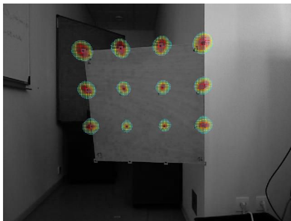
Fig. 4.14: Reconstructed gamma image, representing the position of 12 radioactive hotspots on the experimental phantom, automatically reprojected on the visible image using the intrinsic and extrinsic parameters retrieved by means of the proposed procedure of the optical and \gamma -cameras used.
