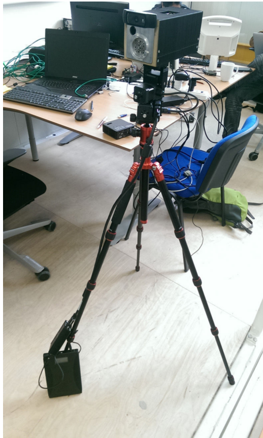
Fig. 3.6: The battery-powered EduPIX \gamma -camera prototype developed for EDUSAFE.
