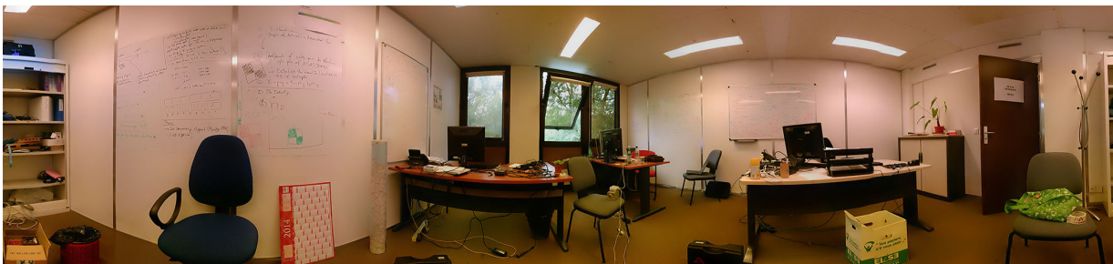
Fig. 3.20: A panorama image with size 7234 \times 1681 pixels captured and generated by the EduPIX prototype, using one single optical camera and a motorized pan-tilt unit, and resulting from the stitching of 80 optical images. The implemented algorithm allows the prototype to autonomously capture high-quality pictures, find and match consistent sets of invariant features, correctly register the images, and compose them together. Clearly, no radiation sources were present in this example. The images that have been stitched together were thus not superimposed by any radiation map in this example.
