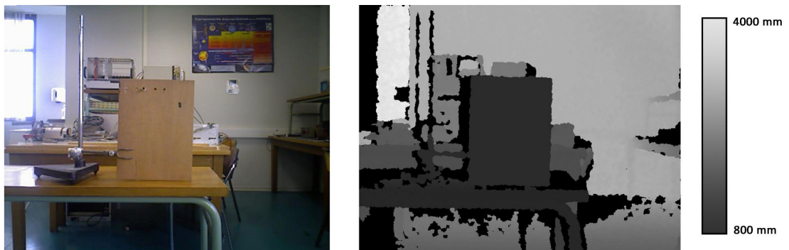
Fig. 4.3: Example of optical image coupled with the respective depth map.
