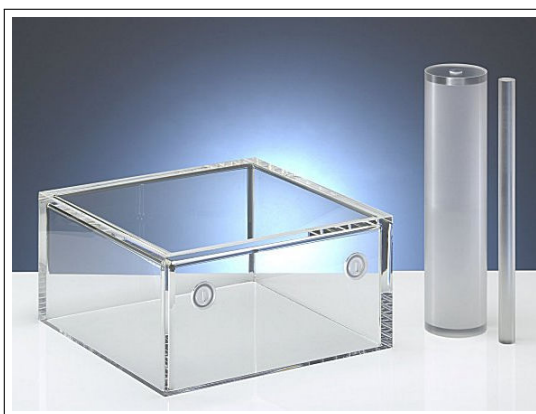
Fig. A.6: ISO phantoms representing parts of human bodies (torso, arm, and finger).
