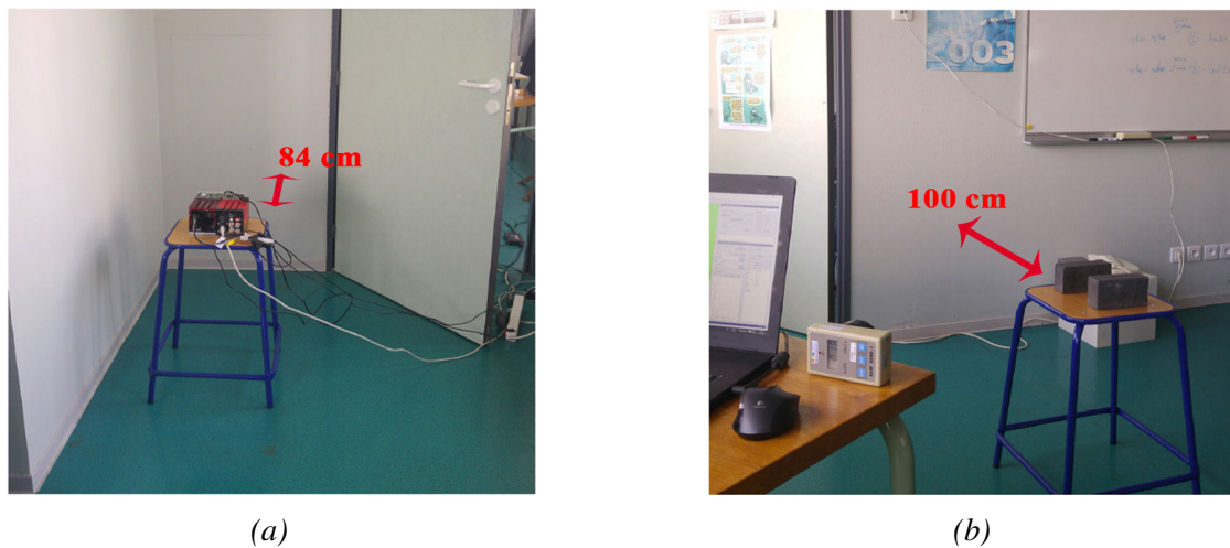
Fig. 4.25: (a) An ^{241}\text{Am} source of \sim 360 MBq activity placed behind a wall while (b) the prototype is on the other side of the same wall, pointed at the source at a total measured distance of 190 cm, and providing an ambient dose equivalent rate of \sim 320 nSv/h at the measurement point.
