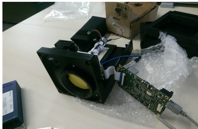
Fig. 4.2: Part of the gamma imaging portable system used for retrieving the 3-D position of radioactive hotspots.
