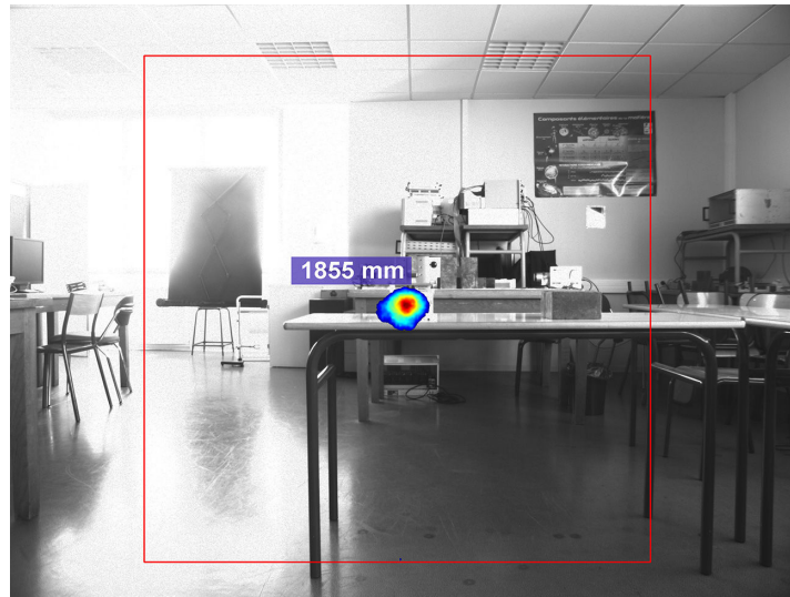
Fig. 4.17: Position and distance automatically retrieved by the prototype for a ^{137}\text{Cs} point source of \sim 261 MBq activity.
