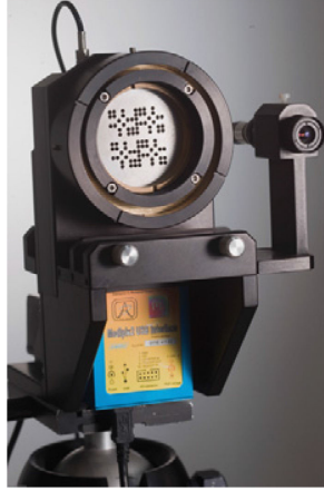
Fig. 1.8: The GAMPIX gamma camera developed by CEA LIST [9].
