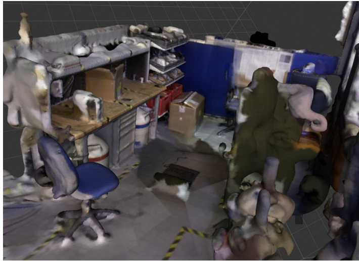
Fig. 4.30: 3-D coloured point cloud representing a CANBERRA laboratory in Montigny-le-Bretonneux, acquired and processed with the prototype. In this example, no radiation sources were present.
