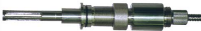
High pressure (20 bar) and temperature (150°C) reflectance probe with a sapphire window; built for operation in corrosive environments
