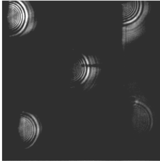
Figure 5.23: Capture of shock waves via lensless AOPDF-based SF-STAMP. Raw image corresponding to the hologram of the object of interest.
