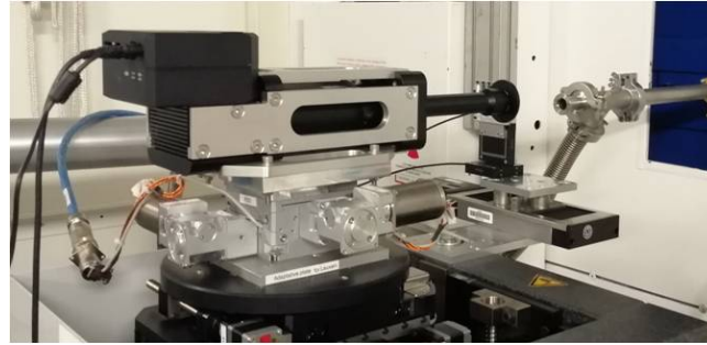
FIGURE 7.19: Picture of the Hartmann X-ray phase imaging system as installed in the BM05 beamline of ESRF.
