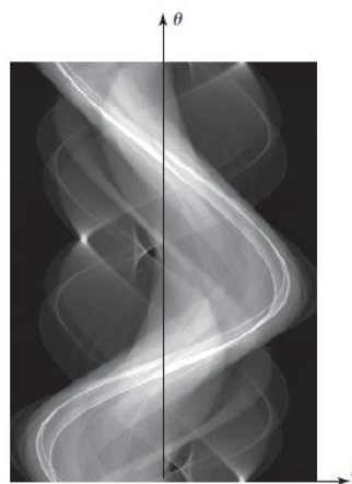
FIGURE 4.4: A sinogram is a 2D dataset p(r, \theta) obtained by stacking the 1D projections p_\theta(r) . Image from (Flower, 2012).
