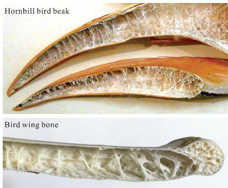
Figure 2.12. Architected cellular structures in the core of bird beaks and bones provide optimum strength and stiffness at low density. [97].
