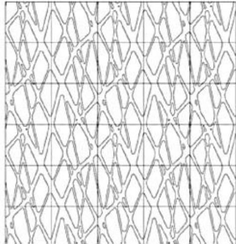
Figure 88 Building E2, the pattern of the exterior metallic skin framing the facade. Source Peripheriques Architectes
