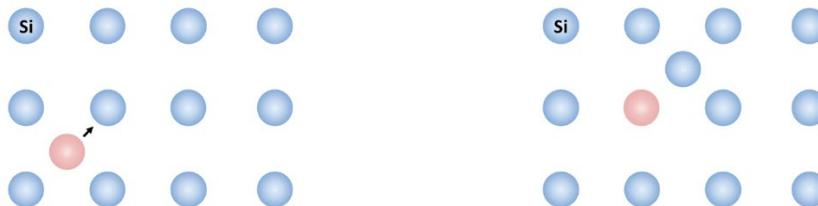
Figure 2.4 Impurity diffusion by the kick-out mechanism
