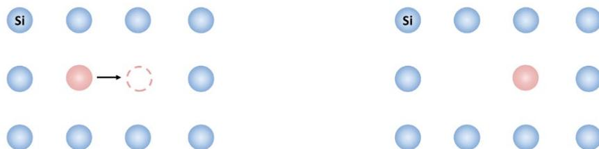
Figure 2.2 *Impurity diffusion by the substitutional mechanism*
