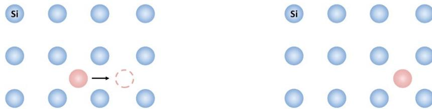
Figure 2.1 *Impurity diffusion by the interstitial mechanism*
