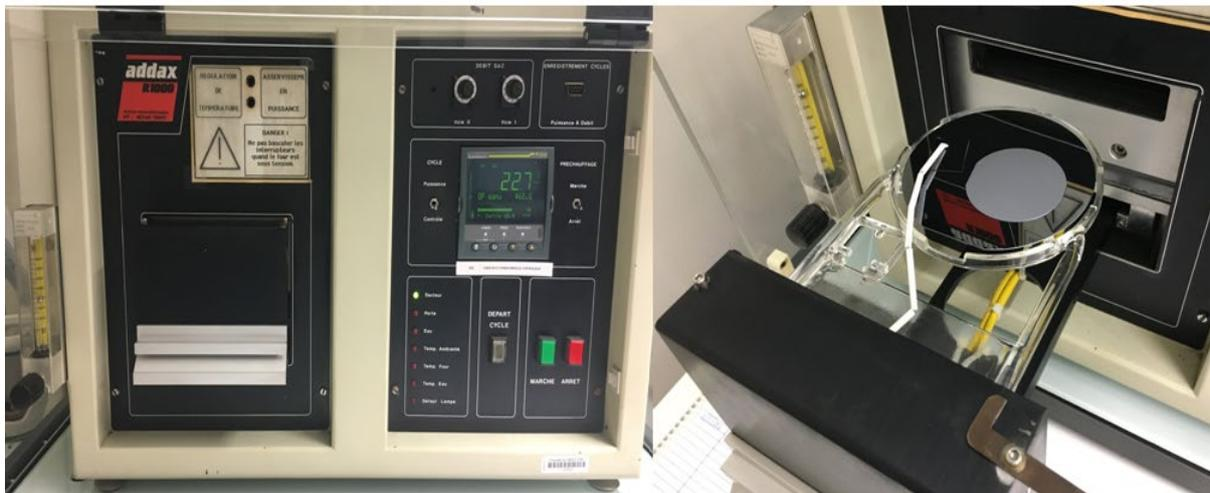
Figure 2.11 ADDAX rapid thermal annealing equipment
