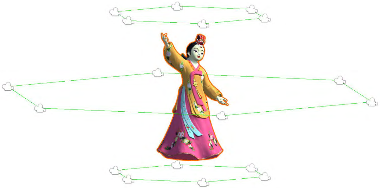
Figure A.11: Camera positions regularly sampled around a 3D object.
