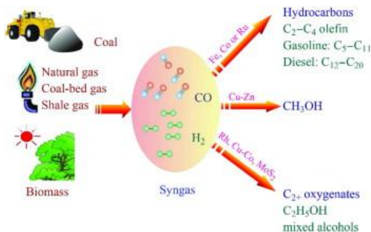
Figure 1.10. Conversion of non-petroleum sources into liquid fuels and chemicals via syngas [61].
