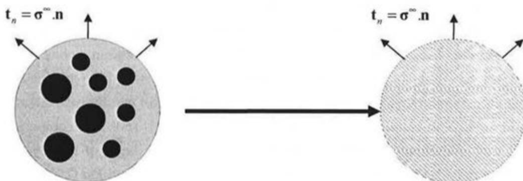
*Figure II.1: Schematic illustrating the replacement of the heterogeneous RVE by an equivalent homogeneous medium.*
