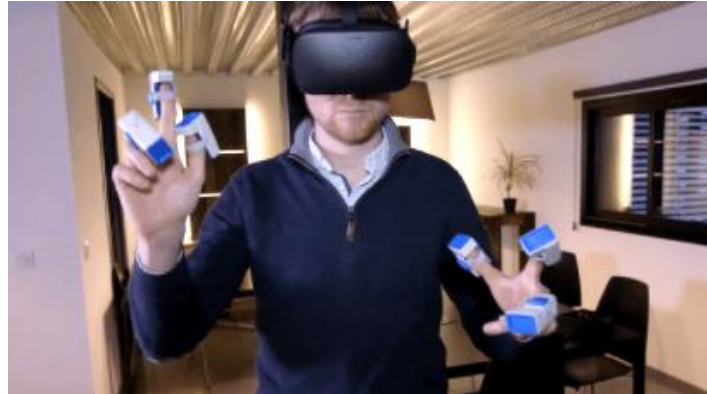
Figure 10. VRtouch: fingertip mounted device for virtual reality [69]
