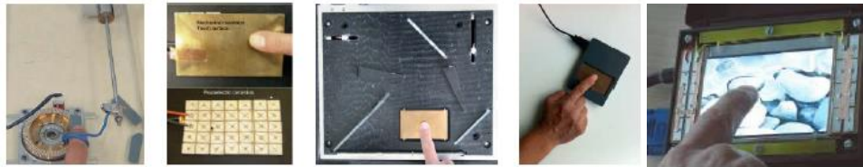
Figure 16. Evolution of the Stimtac prototype: 1D configuration, 2D feedback, 2D input and feedback (2008), compact USB prototype (2010) [30] and transparent prototype (2015) [111].
