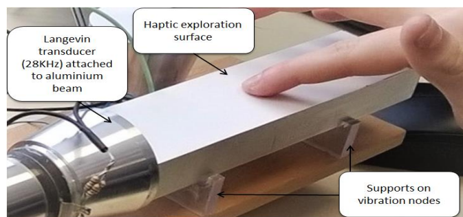
Figure 102. Longitudinal wave haptic device created with a Langevin transducer attached to an aluminum beam
