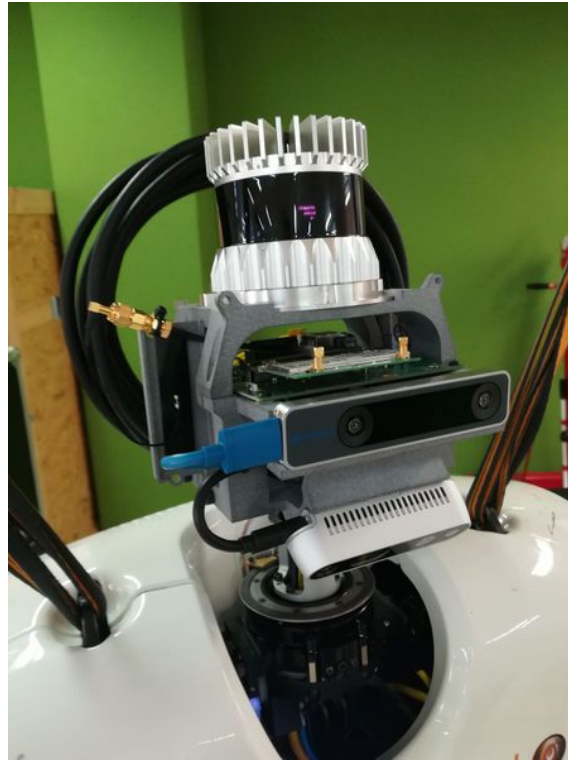
Figure 1.3: Pyrène head with the LIDAR and the two cameras.
