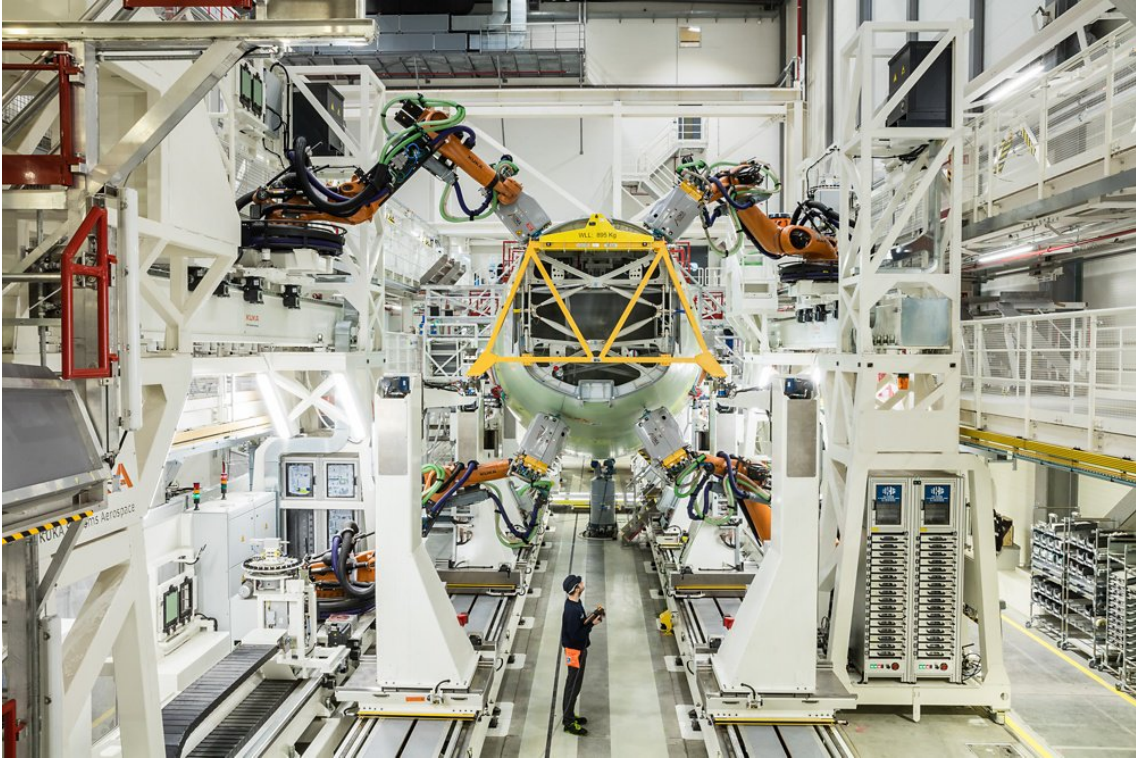
Figure 1.5: Airbus automated fuselage structure assembly line at Hamburg
