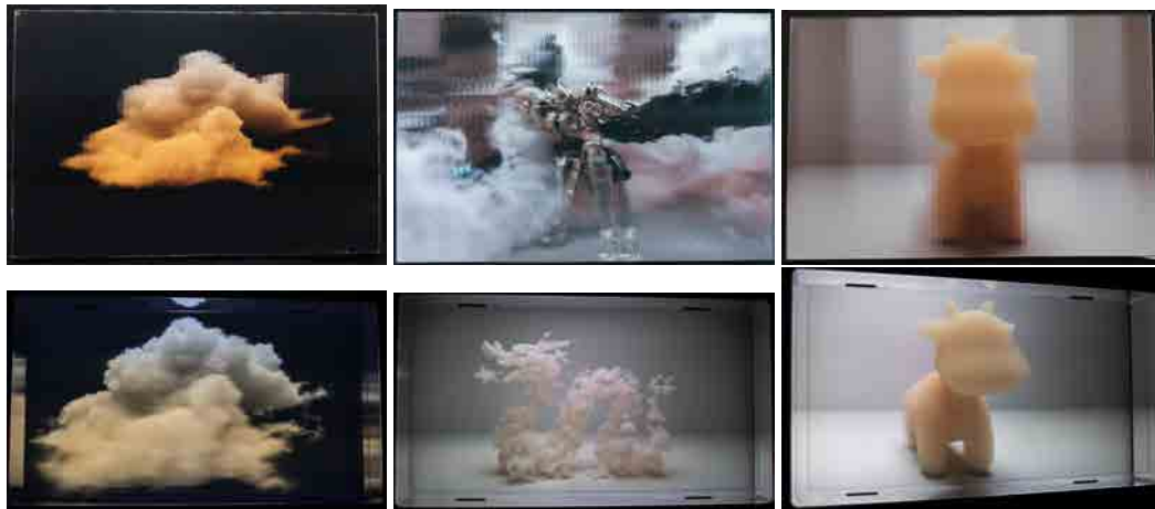
FIGURE 10.3 – Top row. We print lenticular images using 10 views. Bottom row. Our lightfield display renders images consisting of 45 views. We demonstrate our method on 3 light-field images.
