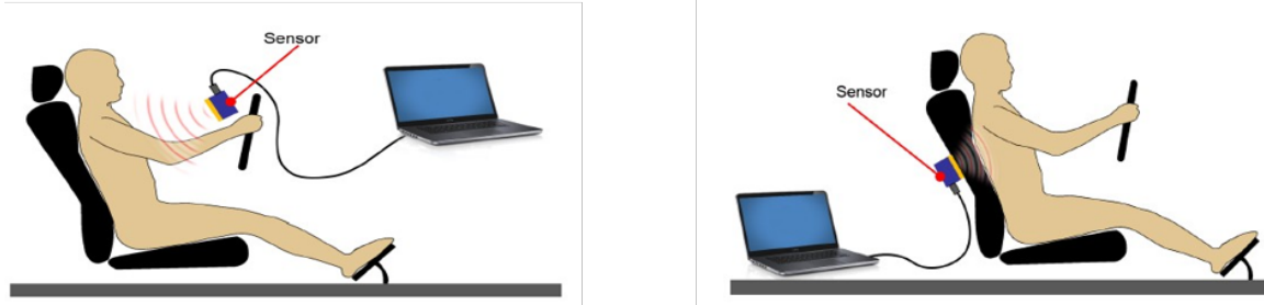
Figure 2.10: (a) The radar is 0.5 m in front of the person, (b) The radar is installed behind the seat [99]
