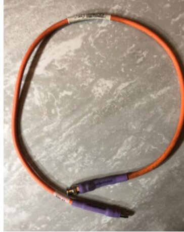
Figure 4.13: The coaxial cable MegaPhase
