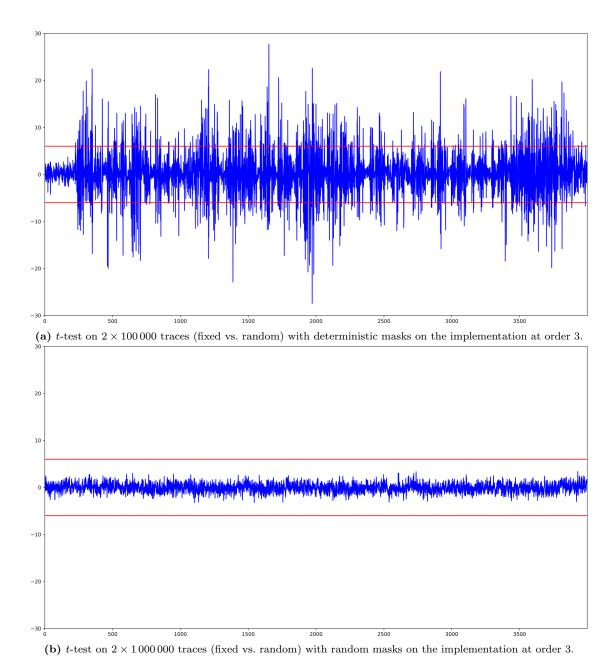
Figure 7.6: TVLA with Welch's t-test on the S-box layer masked at order 3.
