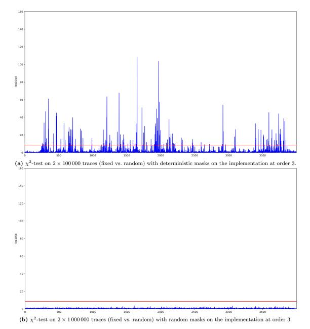
Figure 7.8: TVLA with  $\chi^2$ -test on the S-box layer masked at order 3.
