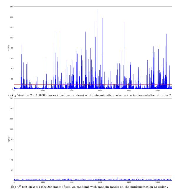
Figure 7.9: TVLA with  $\chi^2$ -test on the S-box layer masked at order 7.
