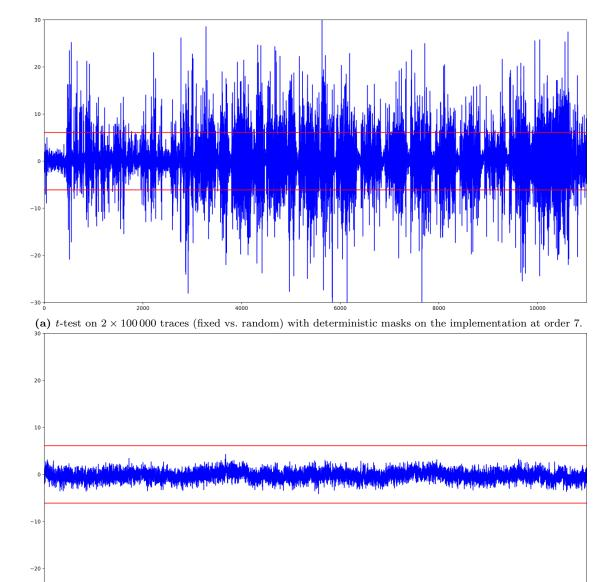
(b) t-test on  $2 \times 1000000$  traces (fixed vs. random) with random masks on the implementation at order 7.
