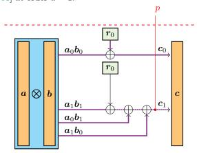
Figure 5.6: Multiplication gadget in presence of hardware glitches.
