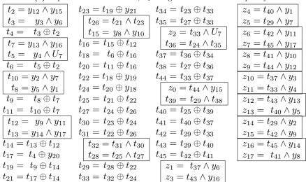
(b) Middle nonlinear transformation with pairs of AND gates highlighted
