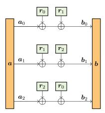
Figure 5.5: Mask-refreshing 2-SNI gadget from [BDF<sup>+</sup>17].
