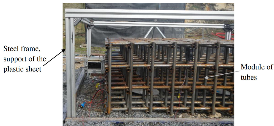
Figure 5.3 – Photograph of the "left" side of the experimental configuration : the steel frame support of the polyethylene sheet, the ignition box and the tubes.
