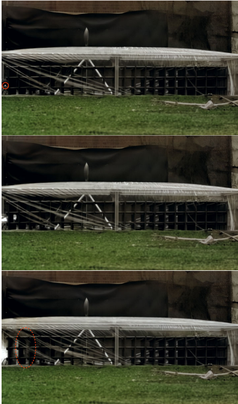
Figure 5.5 – Instant capture by high frequency camera of the early stages of the propagating flame front. Instant depicted are 0.008 s (top) 0.02 s (middle) and 0.06 s (bottom). Flame kernel is identified with plain red circle, area where the flame front is identified but barely visible is identified with dashed red circle.
