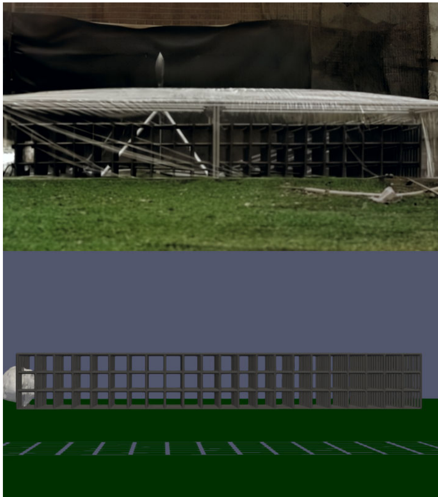
Figure 5.14 – Comparison of numerical (bottom) and experimental (top) flame front, experimental time 0.03 s.
