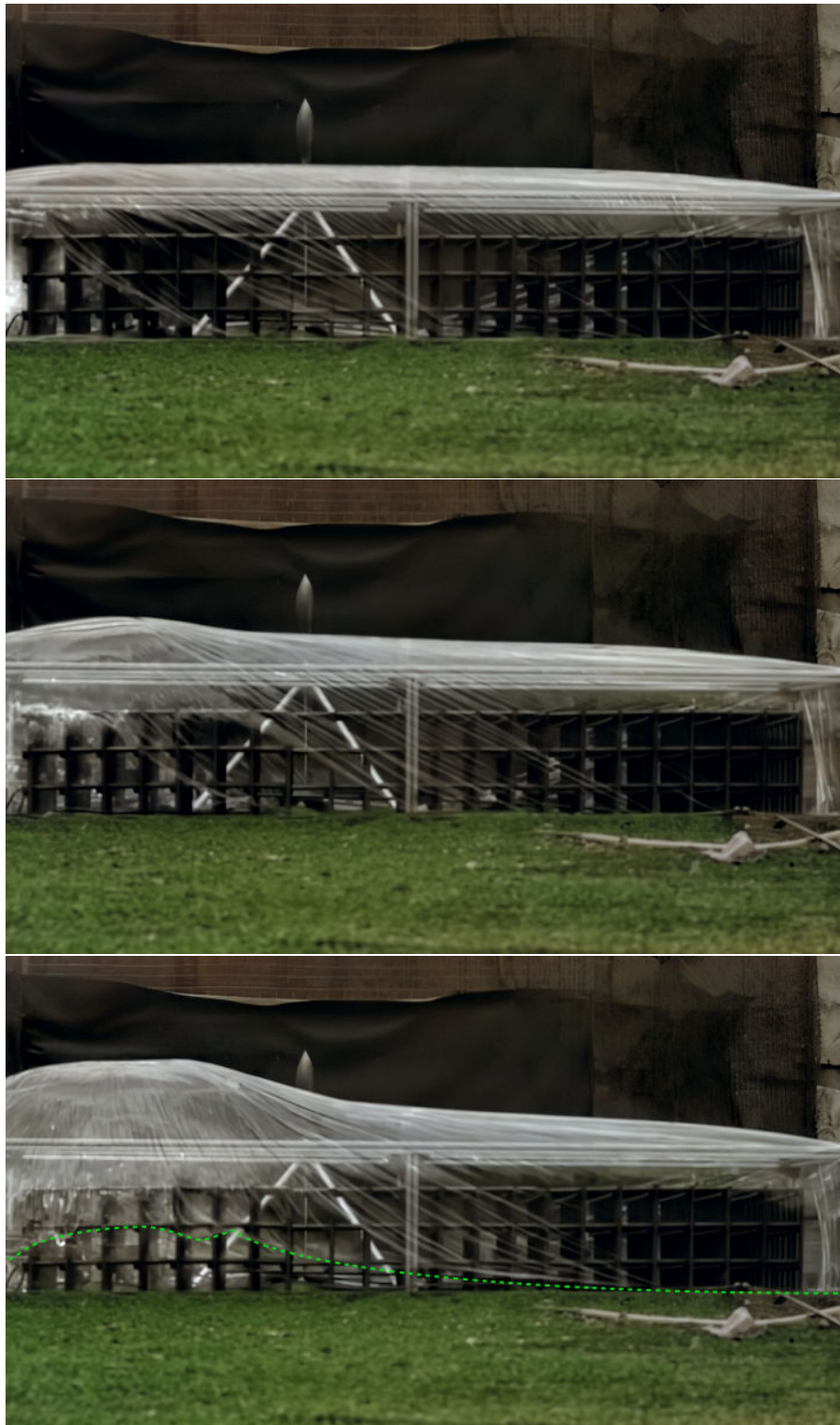
Figure 5.6 – Instant capture by high frequency camera of the propagating flame front. Instant depicted are 0.07 s (top) 0.09 s (middle) and 0.11 s (bottom). Polyethylene film border is identified with dashed green line.
