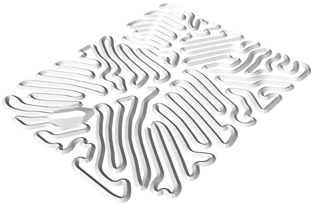
Figure 6.25 Physical model of overlapping deposition and a digital model of a curling path
