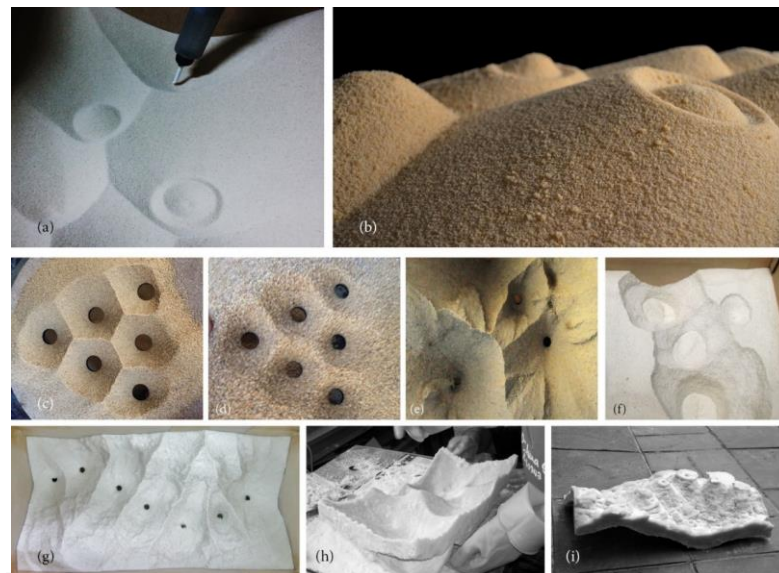
Figure 3.2 Effects of sand characteristics on the emergent patterns. Dry, clean, fine, poorly graded, and rounded grains return sharp ridges and clear surfaces in formation (a) and when solidified (b).
