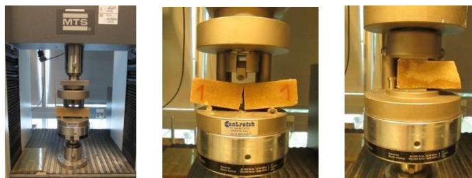
Figure 4.43 Three-point flexural test (left, middle), the compression test on the broken sample (right)
