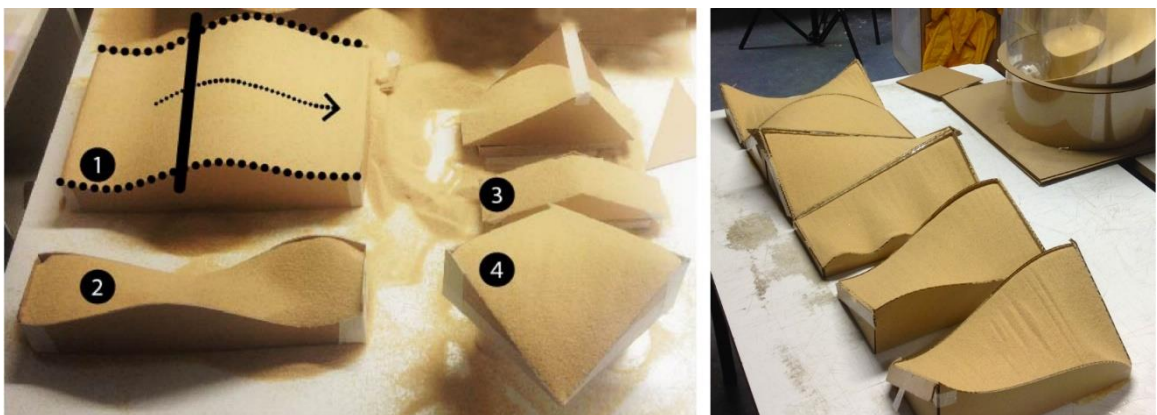
Figure 6.70 Initial experiment of the sweeping formation. The experiment returns single (1,2 - curved & 3- angular), and double ruled (4-Hyperbolic paraboloid) surfaces. Exploration of different typologies (right).
