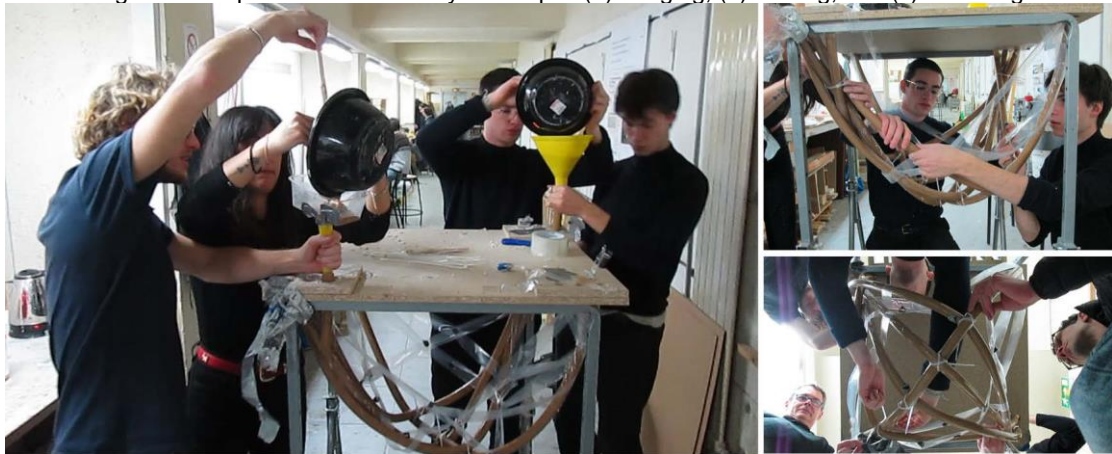
Figure 6.104 The casting process. The model is casted simultaneously from the two ends of the tubes
