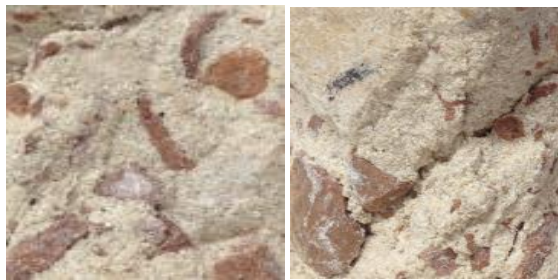
Figure 4.32 Detail of a broken specimen of the mixture of Hyposand and gravel
