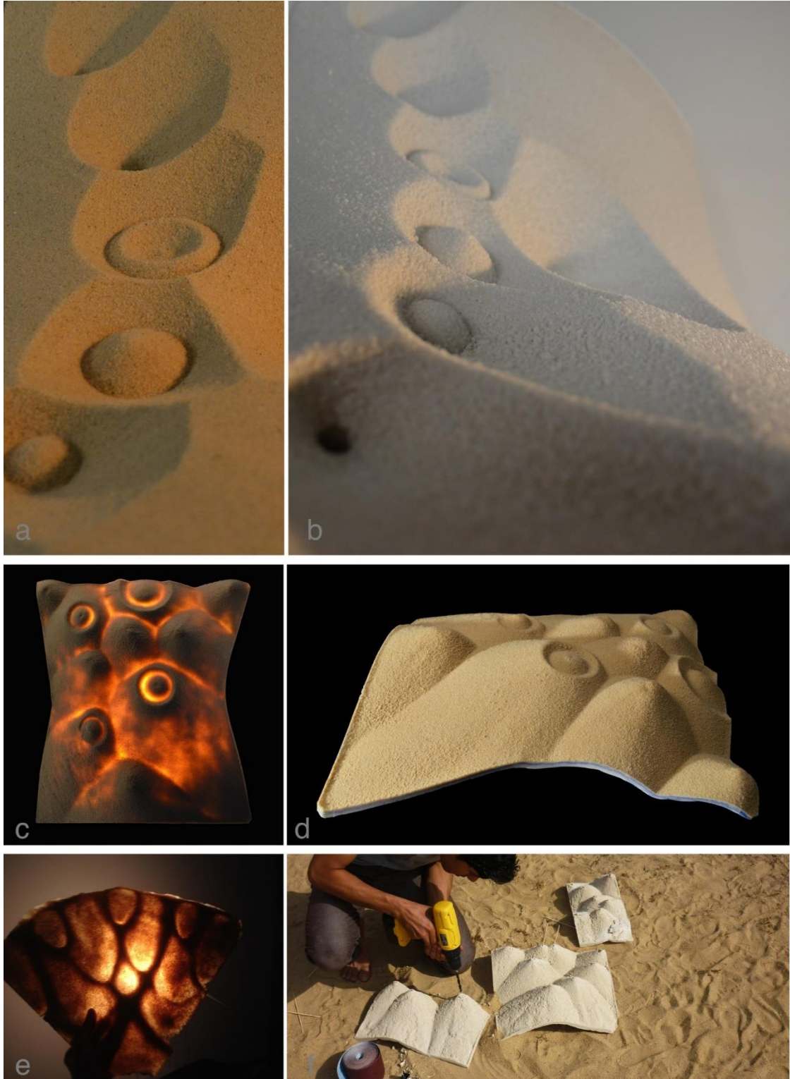
Figure 3.6 Spraying method of making. The precise patterns of loose sand (a) are preserved when solidified (b). A 50x50cm solid panel (d) with a 2 cm thickness border (g). A designed layering of sand allows the development of material translucency (c, e). The resulting panels are strong enough to be worked, drilled transported and casted (h).
