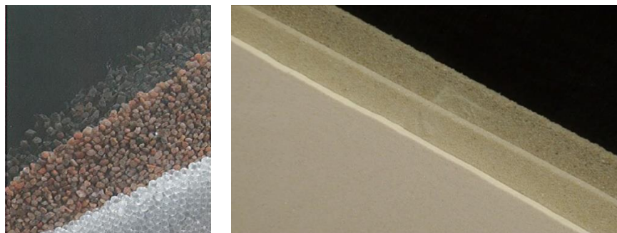
Figure 2.7. The AR of different materials. (Left) the slope of glass marbles (white) is flatter than that of rounded gravels of the same size (red), which is smaller than that of angular gravels (black). (Right) the AR of dry sand is almost the same regardless of the grain size[101].
