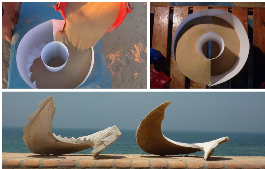
Figure 6.89 First test of helicoid fabrication for a spiral stair design
