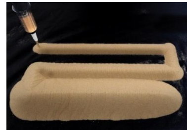
Figure 5.38 Sand deposition methods. Boundary to ridge (left) and ridge to boundary (right).
