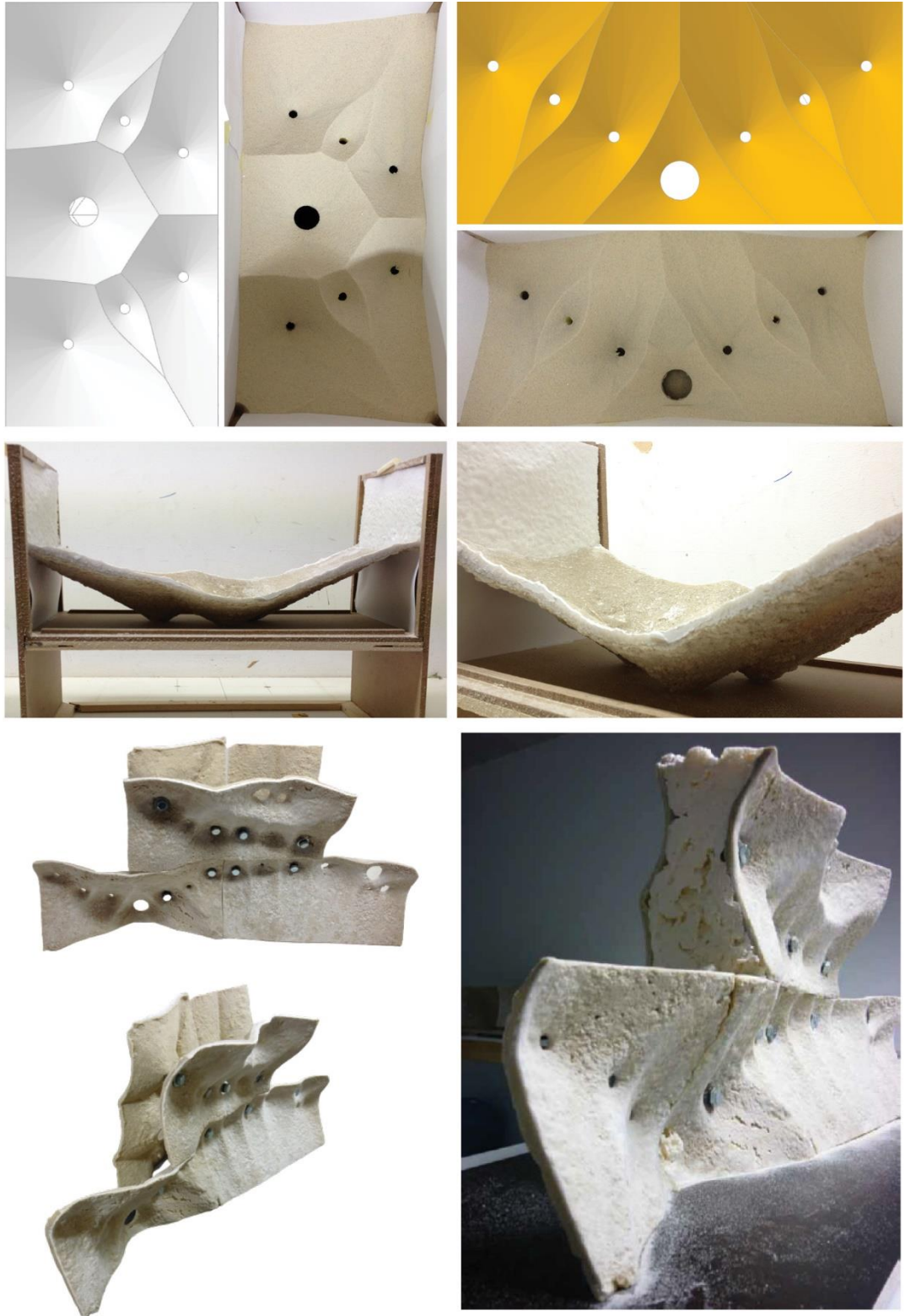
Figure 6.20 Process of making of model D7-12. The model tests the overlapping technique of assembly
