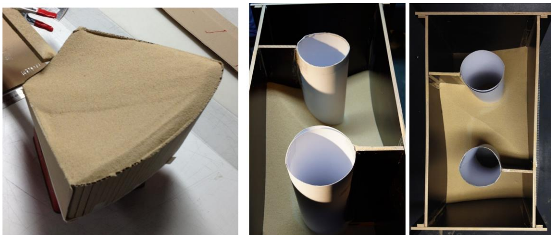
Figure 6.95 Fabrication test of a part of the helicoid surface for larger scale applications (left), and a physical model of a double helicoid 40x80x30 cm (right)
