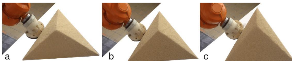
Figure 6.39 The robotic method of tiles formation is based on tilting a horizontal base up to the required tilt
