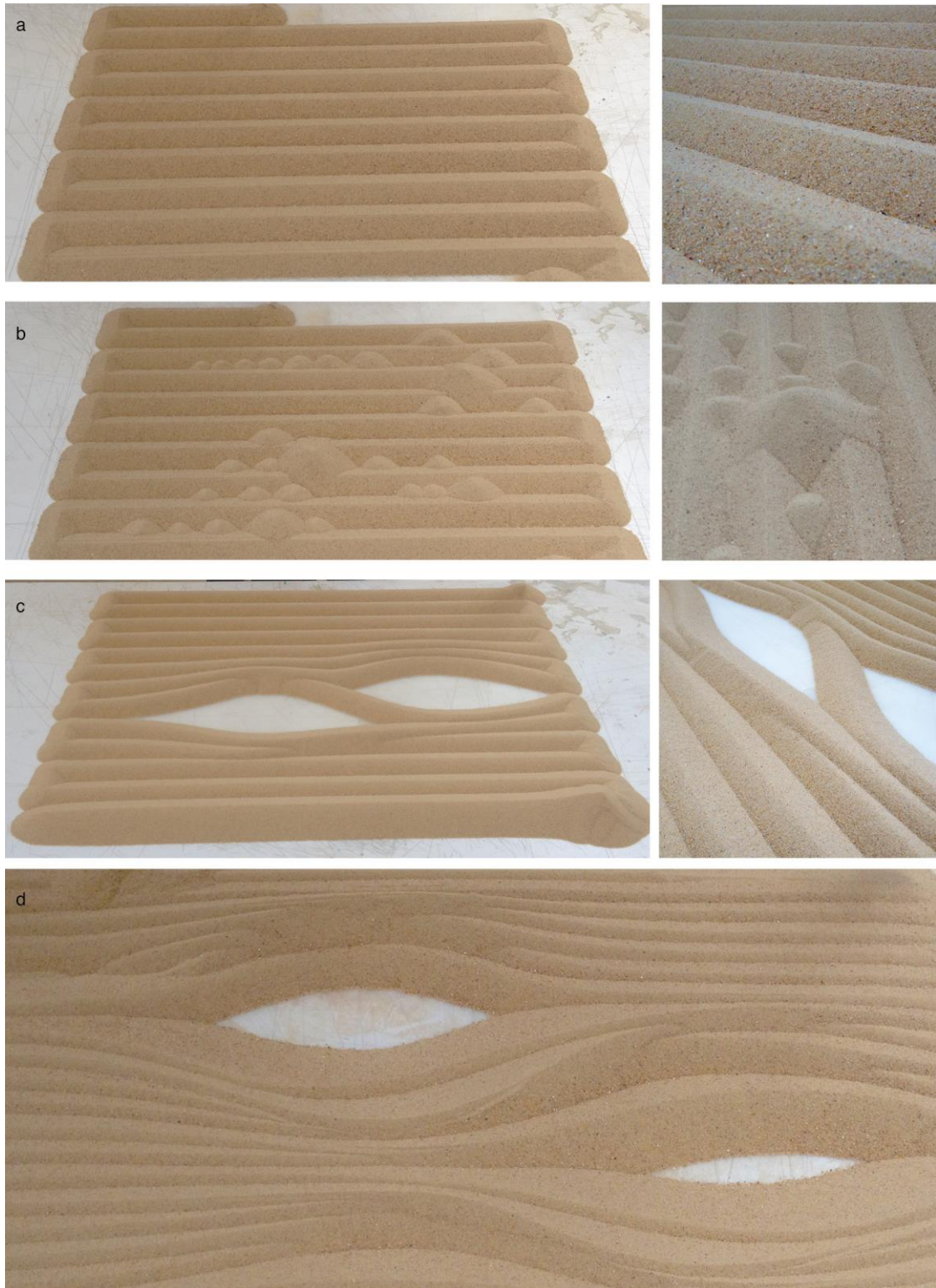
Figure 6.24 Robotic deposition experiments of linear, linear then addition, curved, and overlapping curved paths.
