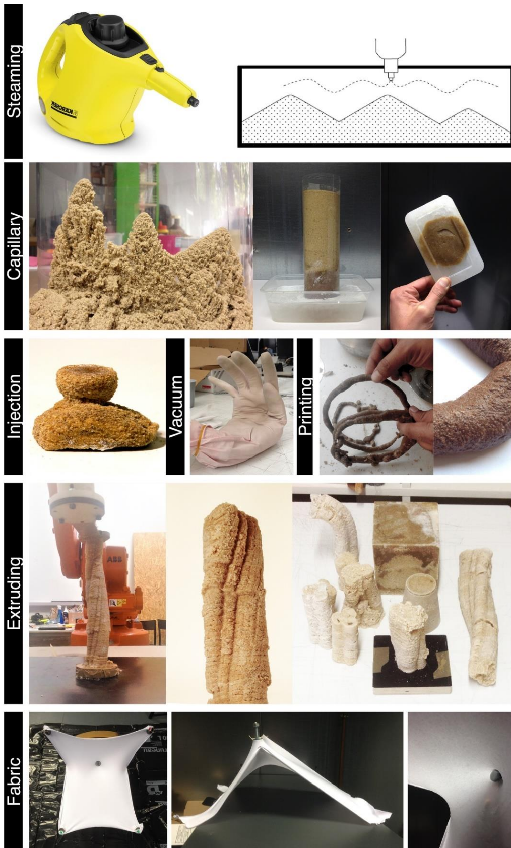
Figure 3.7 Experiments of other making techniques. Mixing sand and salt by: Steaming sand patterns with the saline solution, Capillary action, and injecting salt into sand. Formation of dry sand in vacuum container then injection. Formation of Hyposand by printing and extruding. Solidification of pretensioned fabric by spraying the saline solution.
