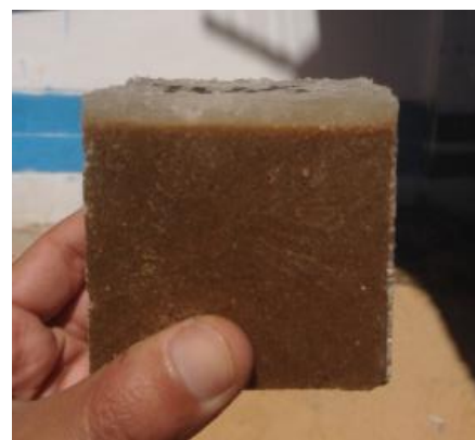
Figure 4.28 The segregation of salt on the top of the specimen.
