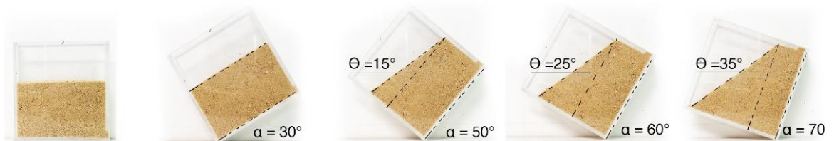
Figure 6.27 Measuring the angle of repose at different tilts
