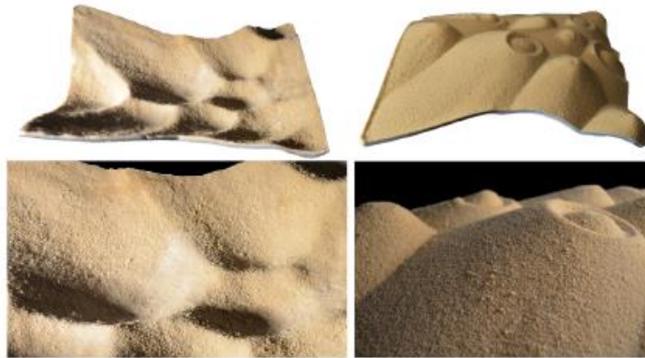
Figure 5.56 the top side (left) and bottom side (right) of a sprayed sand panel.
