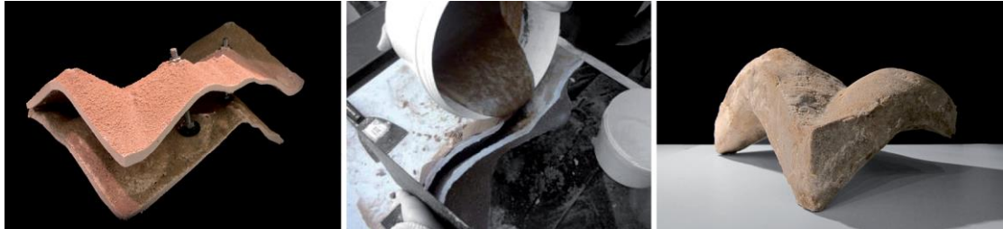
Figure 6.17 The sand block of the 35 Degree project was made of two panels (20x40cm)[1]
