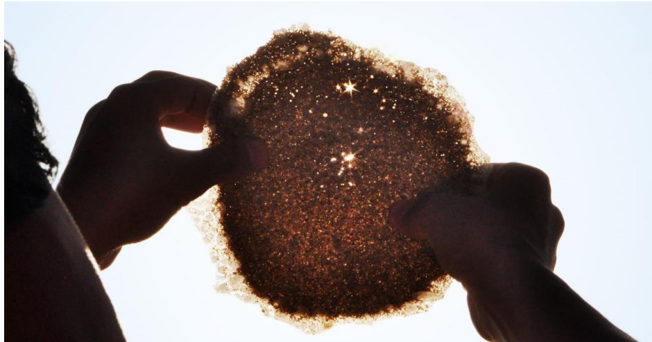
Figure 3.4 A thin crust of sand solidified by spraying
