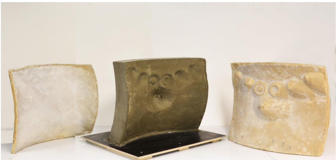
Figure 6.88 Demolded cement block and reusable sand panels
