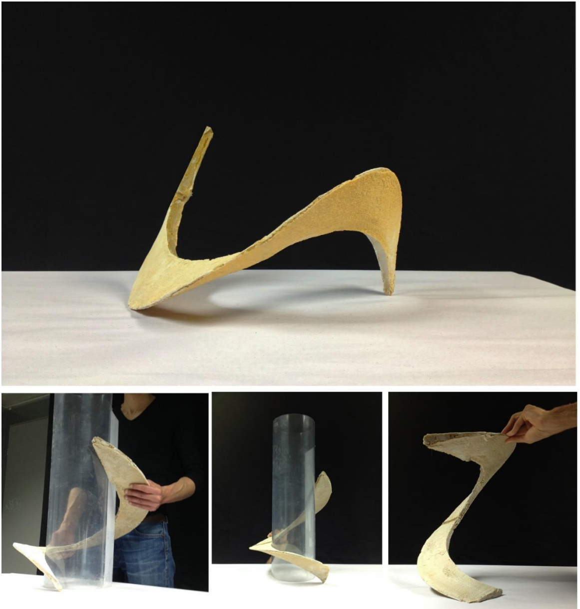
Figure 6.93 Solid helicoid surface made of sand. (height 30cm, radius 25cm, thickness 2cm)
