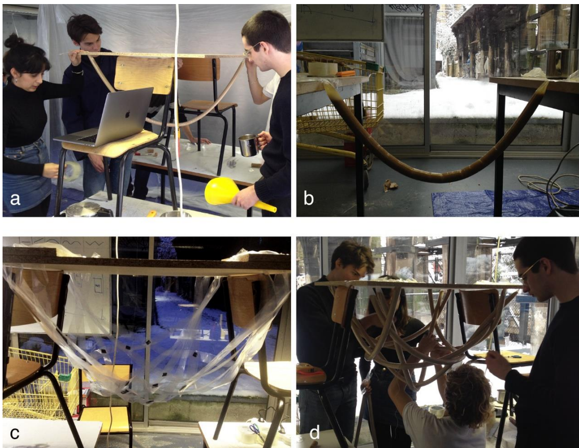
Figure 6.102 Initial test to determine the catenary curve and the technique of making. (a) dry sand, (b) wet sand, (c) hanged plastic sheaths, and (d) organization of dry sand tubes.
