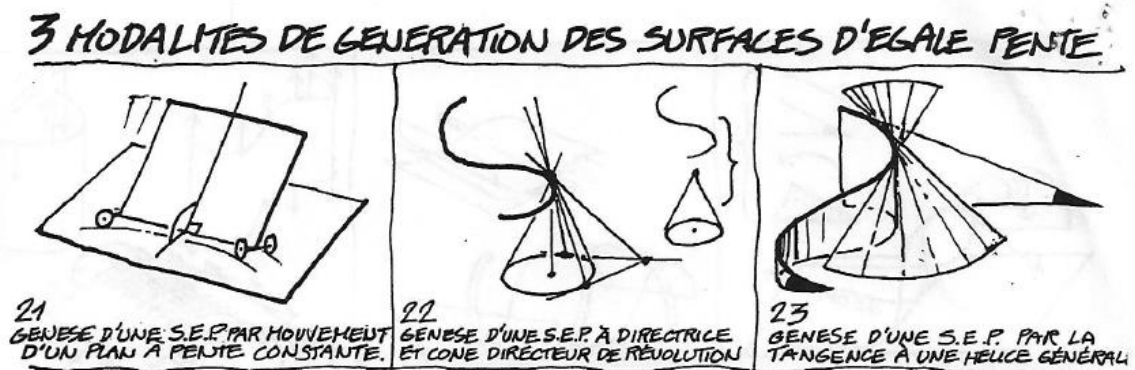
Figure 2.12 Methods of generation of surfaces of constant slope [69,70]
