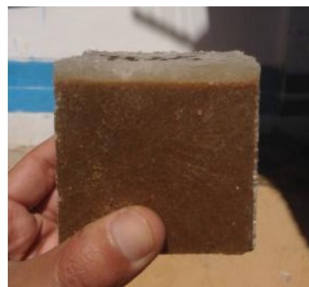
Figure 4.28 The segregation of salt on the top of the specimen.
