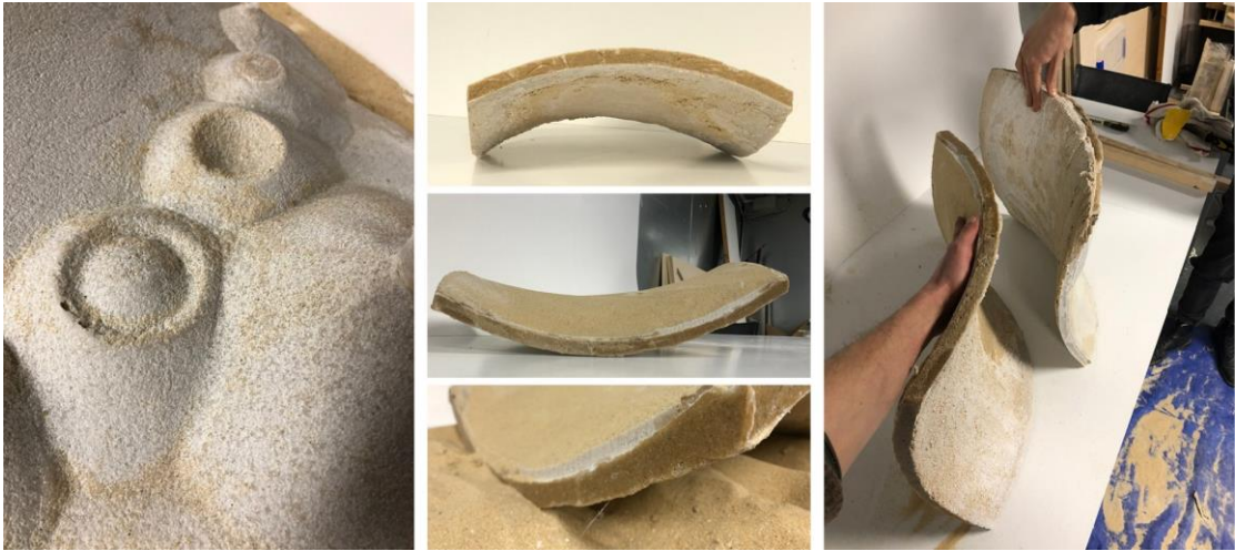
Figure 6.86 Details of the panels ridges and edges
