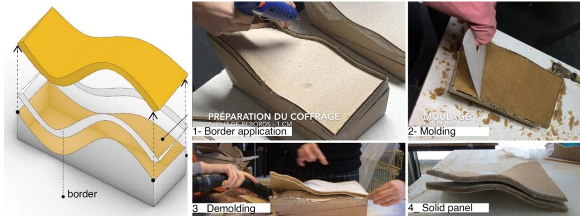
Figure 6.72 Initial experiment of the sweeping technique of fabrication. The developed formwork is composed of a box and a border (left). The procedure of making a panel (right)
