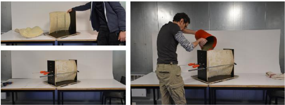
Figure 6.87 Assembly and casting of the panels with cement
