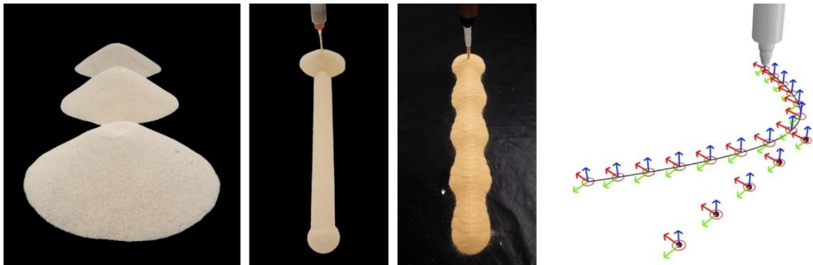
Figure 5.50 Tests of tuning the robot speed and wait duration with the flow of sand and the resulting heights.
