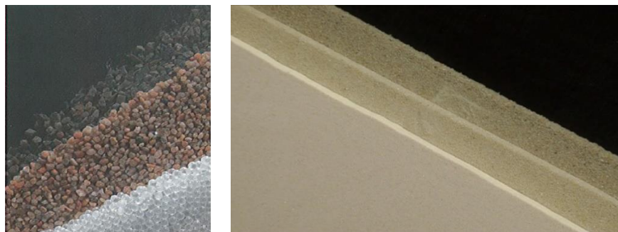
Figure 2.7. The AR of different materials. (Left) the slope of glass marbles (white) is flatter than that of rounded gravels of the same size (red), which is smaller than that of angular gravels (black). (Right) the AR of dry sand is almost the same regardless of the grain size[101].
