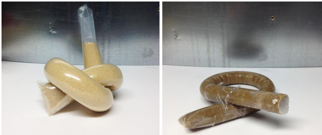
Figure 6.99 Formation of sand tubes: dry sand (left) and solidified and (right)
