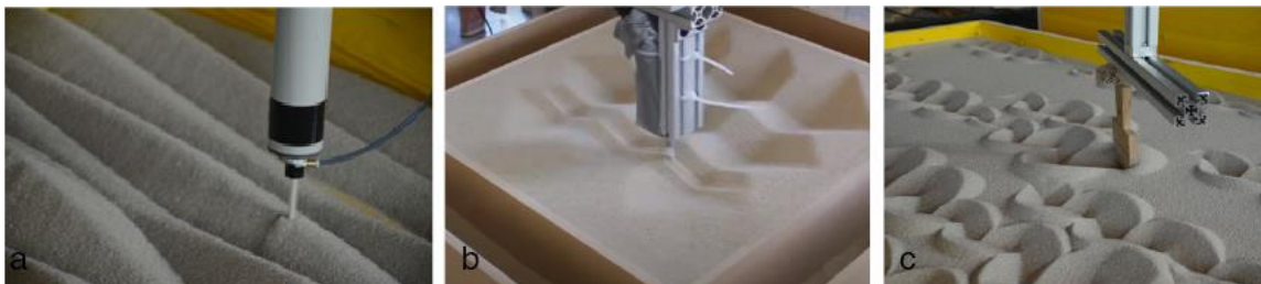
Figure 1.15 Robotic sand forming techniques. (a) deposition, (b) subtraction, and (c) displacement [66].
