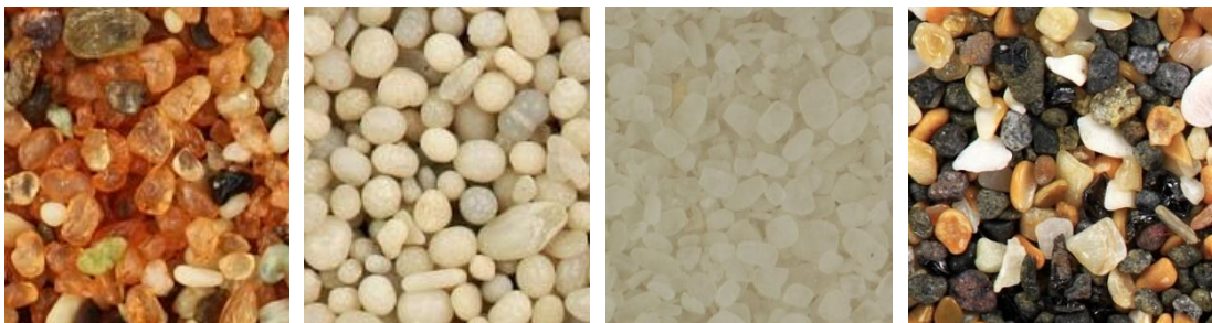
Figure 2.1 Visual assessment of sand type. From left to right: desert silica, coastal carbonate, desert gypsum, and beach biogenic (a mixture of organic and silica). [86]
