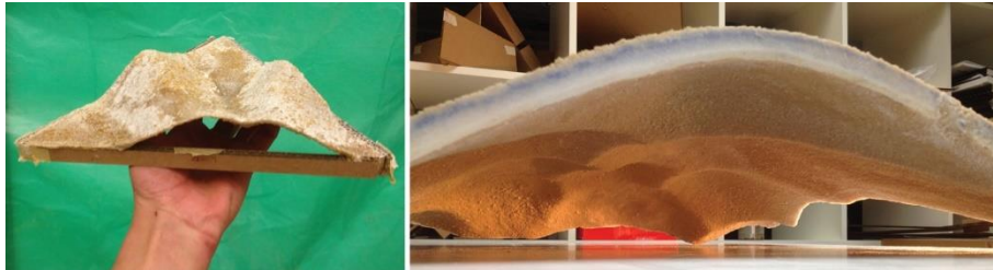
Figure 5.53 The size of panels is restricted by its thickness and the feasible size of the formwork. A 0.3cm thickness for a 20 cm panel (left), and 20 mm (right)
