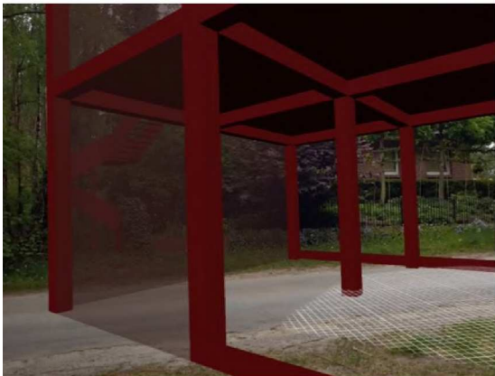
Figure 6. Virtual immersion into the 3D model of La Folie N.5, in a different location from the Parc de la Villette. Verifying the limitations of AR in terms of natural lighting. More adjustments in brightness needed.
