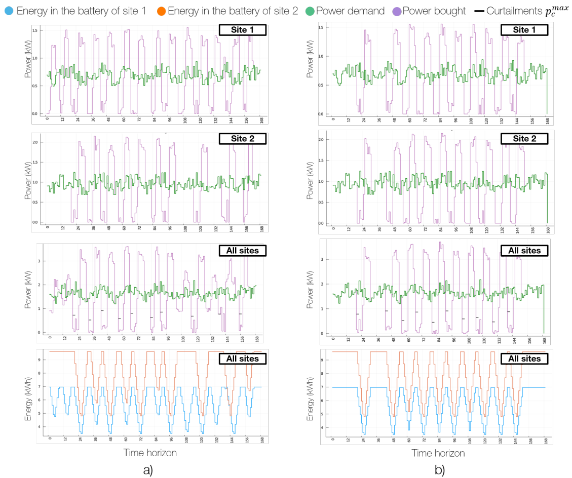
Figure 5.4 – Solutions obtained with (a) CPLEX solving the ( OMBSE - MILP ) model, and (b) with the Lagrangian relaxation for an instance with 2 sites managed over a week.
